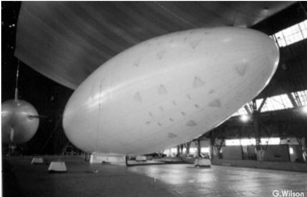
StratSat's bare helium filled envelope was held down by heavy concrete blocks in a hanger at Cardington. The many triangular anchor points on the envelope mark locations that may carry a load. Source: Grahame Wilson via The Airships at Cardington, UK
