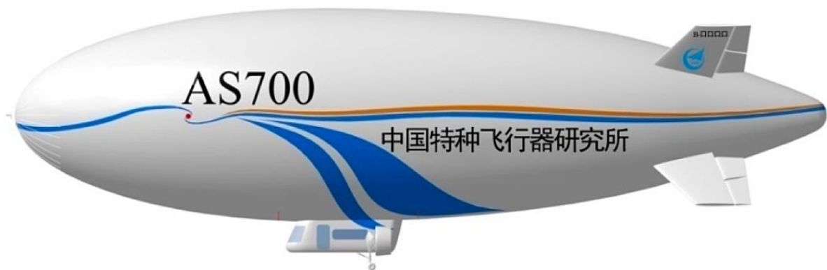
AVIC AS700 non-rigid airship. Source: AVIC Special Vehicle Research Institute
