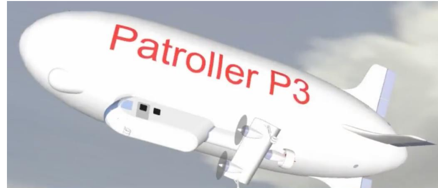
Note the X-tail with active control surfaces. All three engines are mounted behind the gondola.
