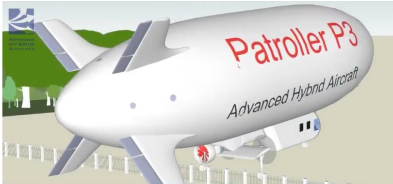
Note the X-tail with active control surfaces. All three engines are mounted behind the gondola.
