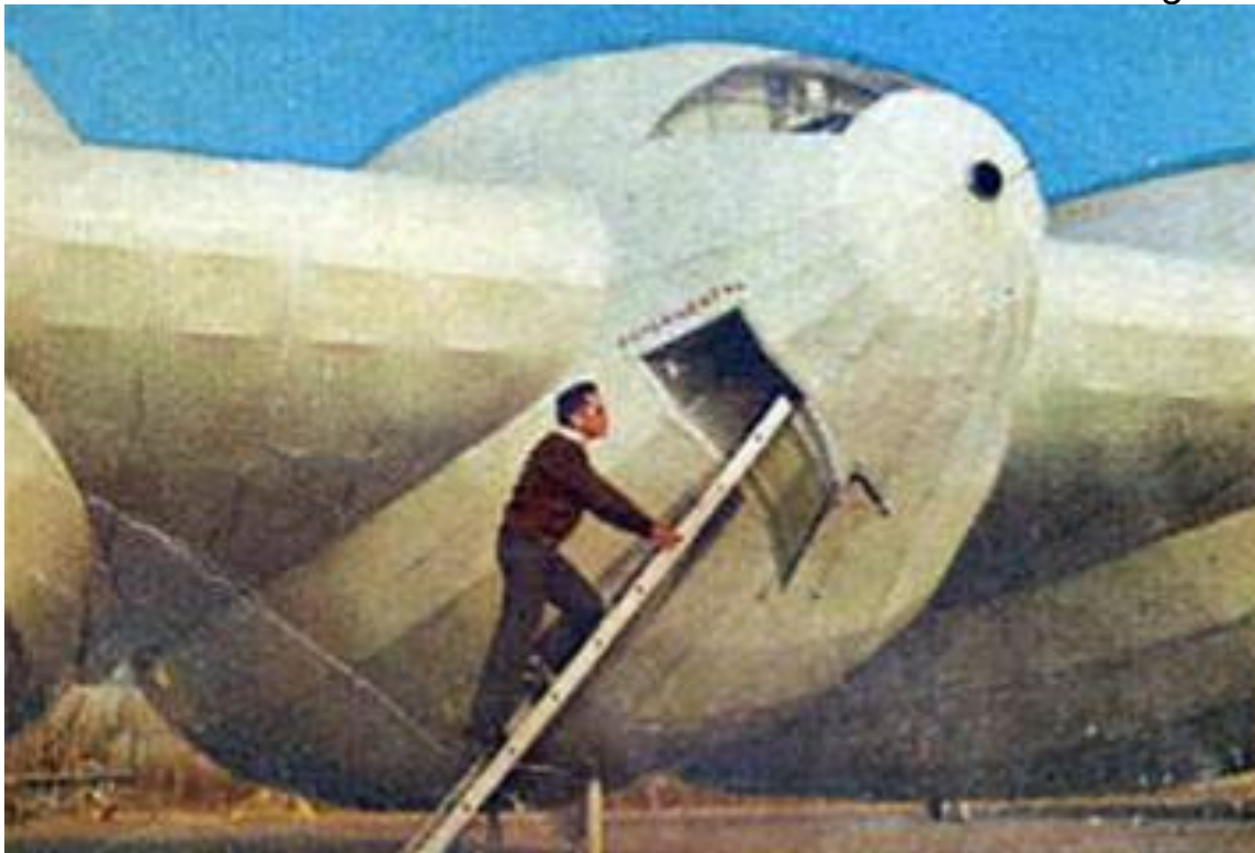
Aereon III showing crew access into the central hull. Source, both photos: Nigel Kaley, 2003
