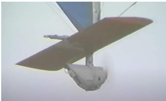
Closeup of a wing airfoil and engine unit on the tip of a blade airfoil. Source: Screenshot from Rob Crimmins video
