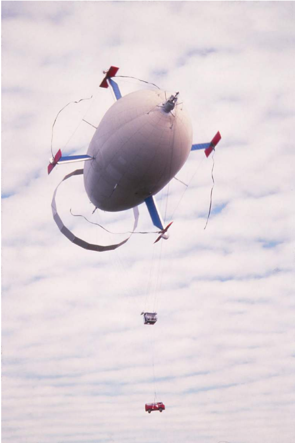
The rebuilt Cyclocrane in flight. The crew cab is suspended beneath the aerostat and a 1-ton VW minibus is attached as a sling load. Source: Rob Crimmins
