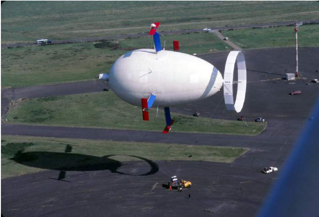
The rebuilt Cyclocrane. The wing airfoils are red, the blade airfoils are blue. Source: Rob Crimmins
