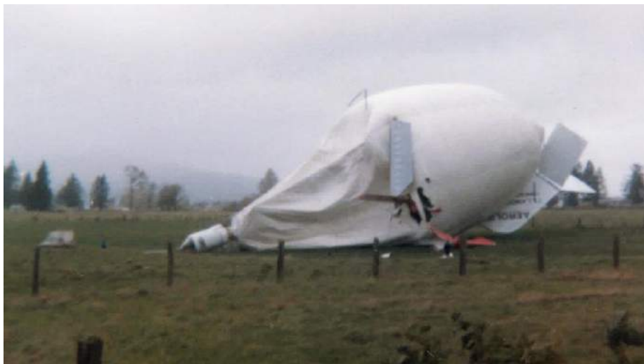
The original Cyclocrane after breaking free from the mast during a storm, 23 October 1982. Source, both photos: Rob Crimmins
