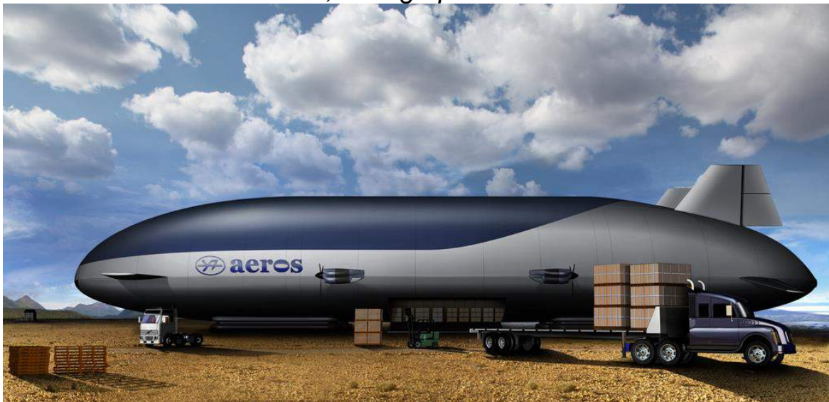
ML866 / Aeroscraft Gen 2 ground cargo handling. Note the side access to the cargo bay. Source, both graphics: Aeros
