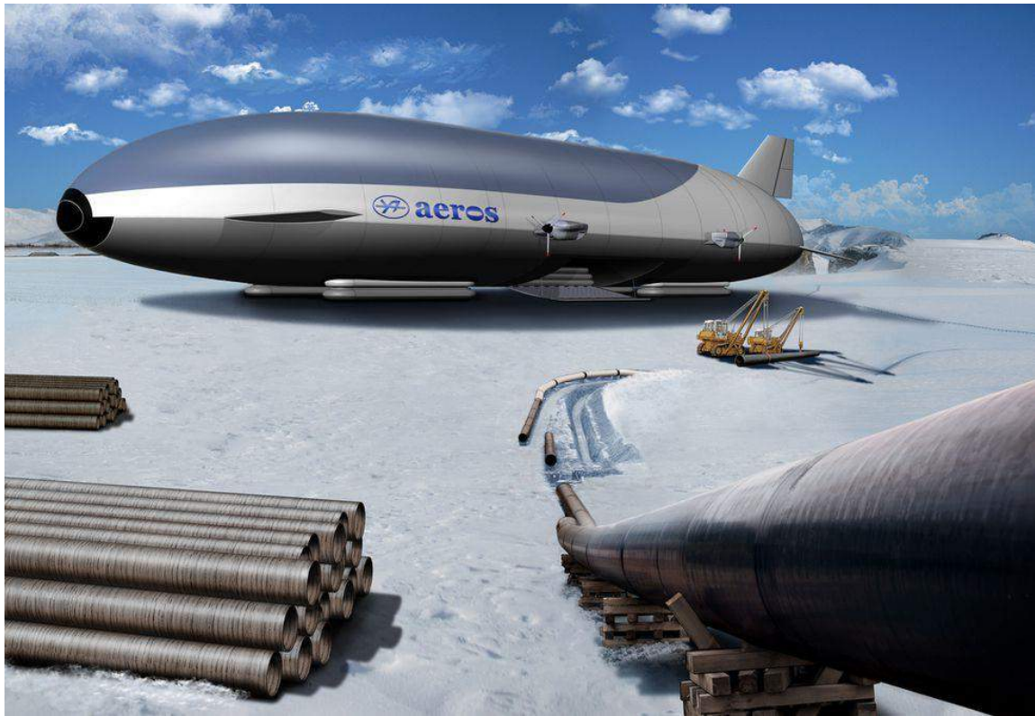
ML866 / Aeroscraft Gen 2 ground cargo handling. Note the side access to the cargo bay. Source, both graphics: Aeros
