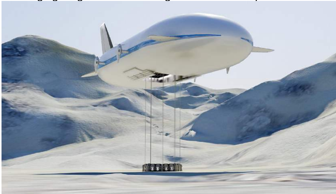
ML866 / Aeroscraft Gen 2 hovering and making an in-flight load exchange. Source, both graphics: Aeros
