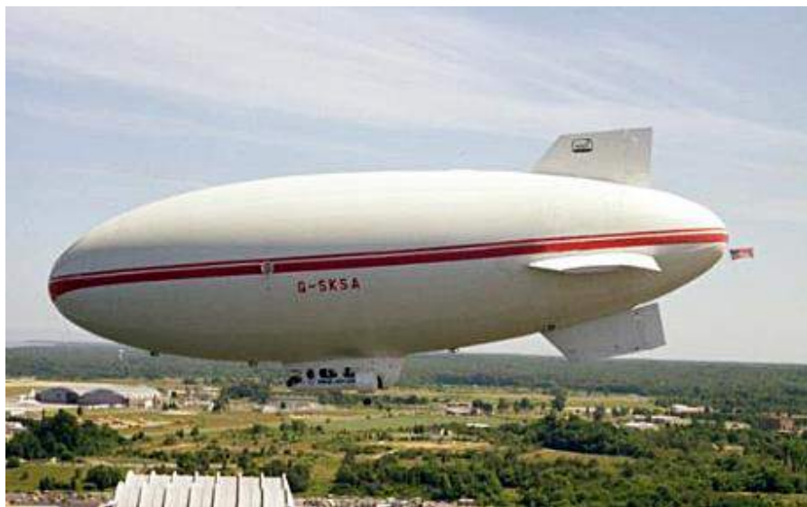
Skyship 500 flying in 1983 US Naval Air Development Center test of airship flying qualities, performance, and radar cross-section. Source: Wikipedia
