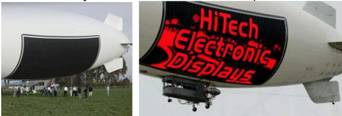
The 70 x 30 foot Video Lightsign blank screen (left) and in operation (right). Source: Technovelgy.com (2006)
