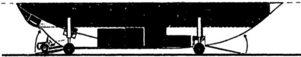
Side view of the Helitruck payload bay open at both ends. Source: UNIDO, Section 7.5 (1983)
