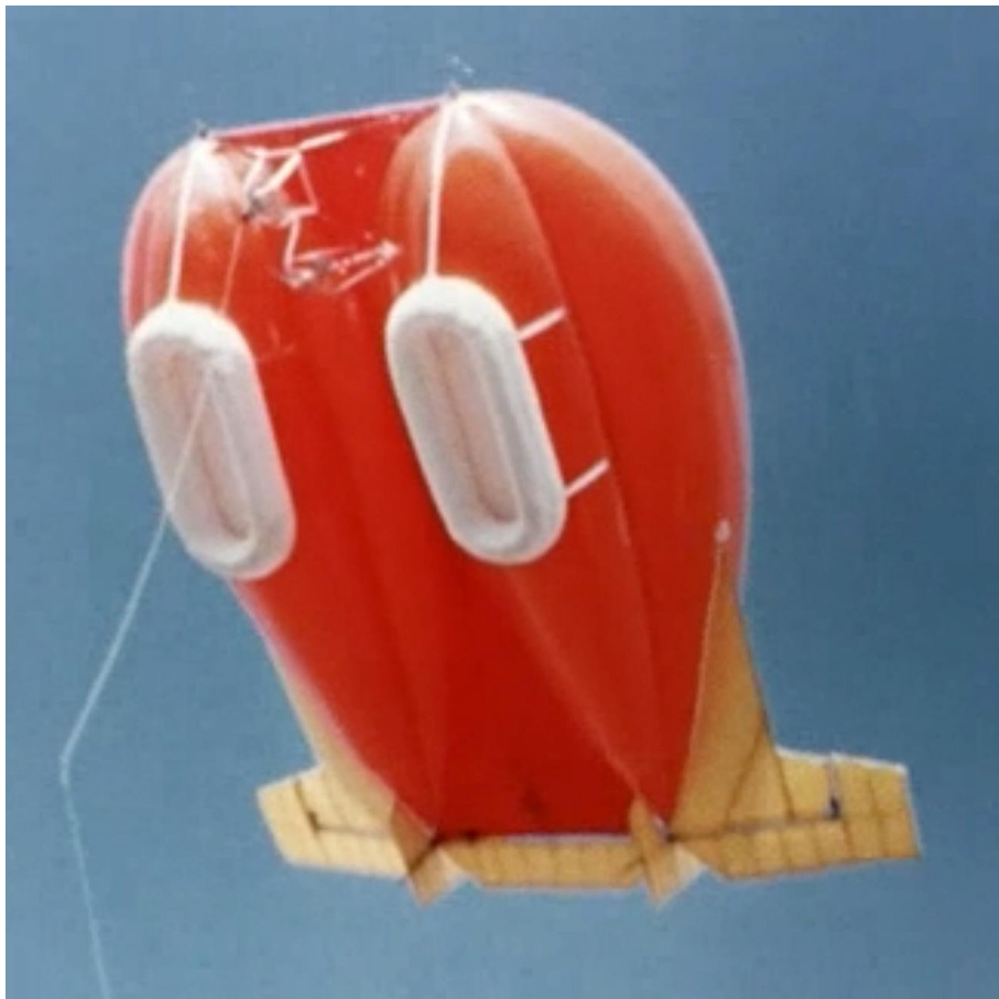
Underside showing the white ACLS pods, the engine positioned at the front of the central “tunnel” and the rear wing and control surfaces.
