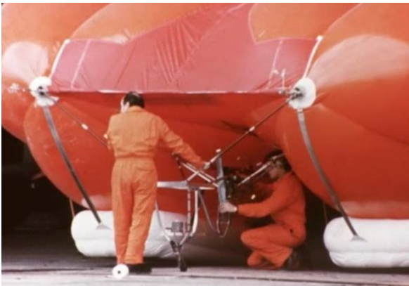
Engine installation in the tunnel between the catamaran hulls.
