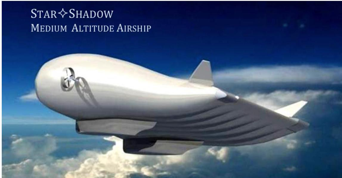
*Renderings of the StarShadow hybrid airship in flight. Note the two widely spaced gondolas (above), the flexible, thin-film photovoltaic array on the top of the hull (below), and the flank-mounted, thrust vectoring, ducted fan main propulsors. Source, both graphics: ENSS*
