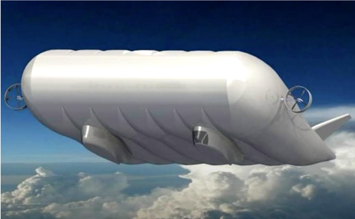
Renderings of the StarShadow hybrid airship in flight. Note the pilot-optional cockpit in the port gondola (above). Also note the seven lobes in the broad lifting body envelope (below) and the flexible, thin-film photovoltaic array on the five central lobes. Source, both graphics: Screenshots from GNSS 2010 video.
