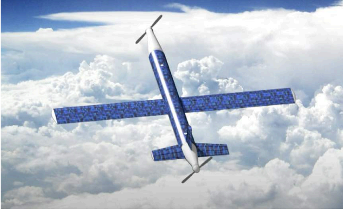
StarLight SRV with extendable wing solar panels stowed (during ascent & fly-down).
