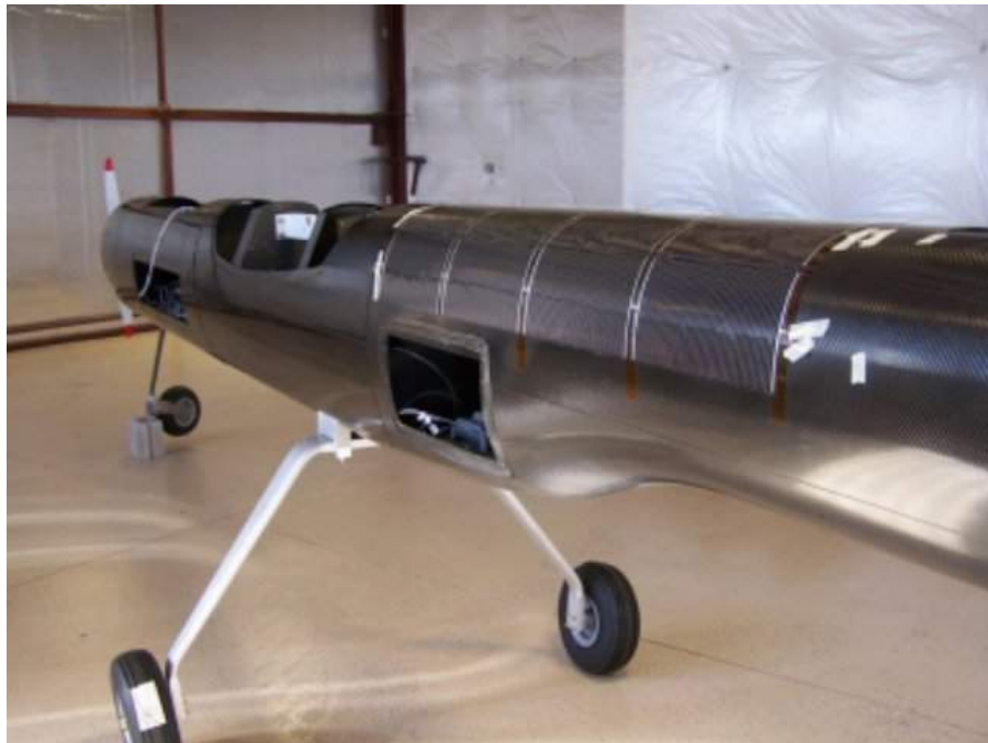
Rear quarter view of the partially complete fuselage for the 40%-scale SRV demonstrator. Source: UAS Vision
