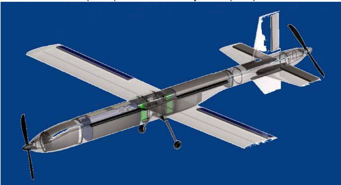
General arrangement of the StarLight SRV (the Fly-Down Lower Stage) with its solar panels deployed on station (above) and retracted during the fly-down (below). Source: Enerbay - NSS (2015)
