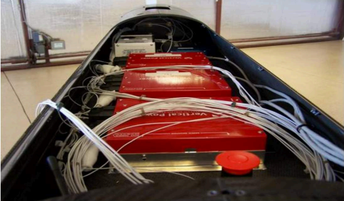
Battery packs in the partially complete fuselage for the 40%-scale SRV demonstrator. Source: ENSS
