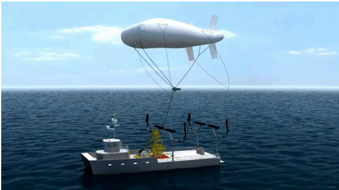
Concept for StarTower tethered aerostat deployment from a small utility vessel. Source: Screenshot from Deep Down Inc, video (2014)
