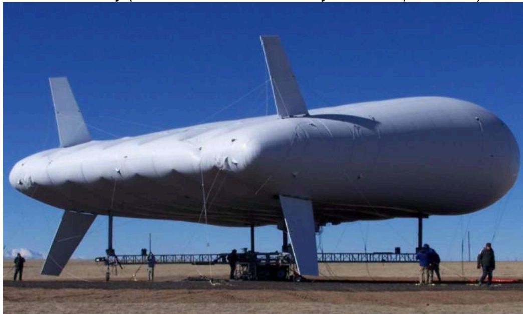
General arrangement of a SkyTower operating base. The winch is on the Base Station (center). The system can be operated locally (at the Base Station) or remotely (from the Ground Control Systems & Ops Vehicle).
