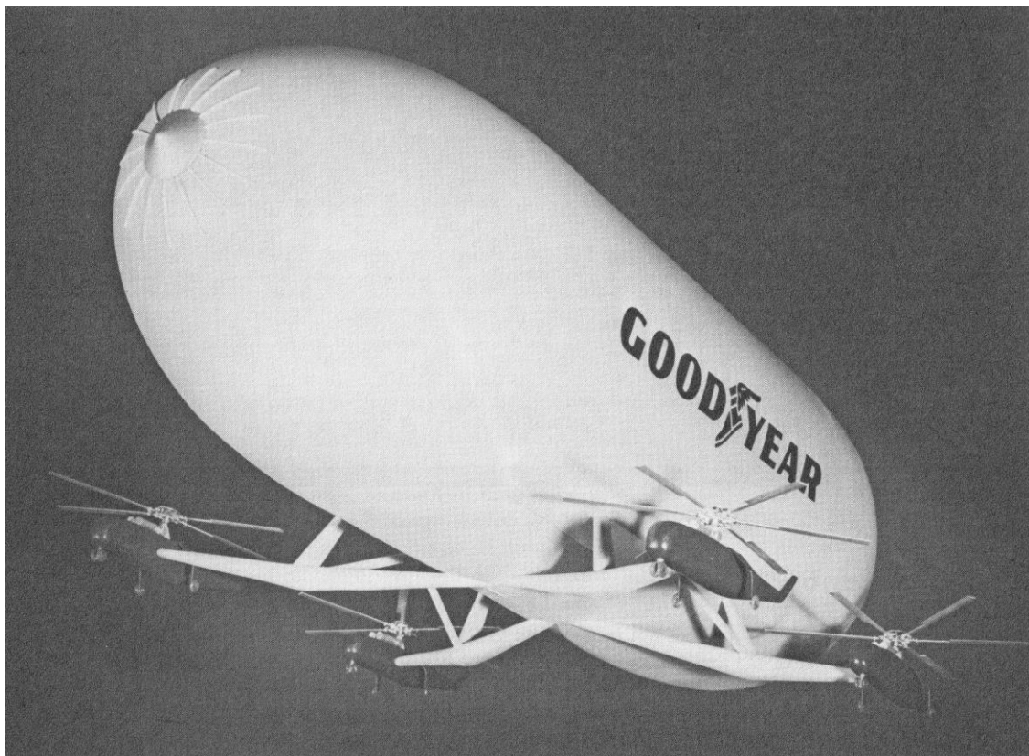
A model of the initial Goodyear Aerospace HLA helistat design concept circa 1976, with four CH-53B helicopters mounted on rigid frames under the gas envelope. Source: Goodyear Aerospace via Airships for the Future (1976)
