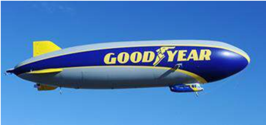
Goodyear’s new “blimp” – a semi-rigid Zeppelin LZ N007-101. Source: Goodyear
