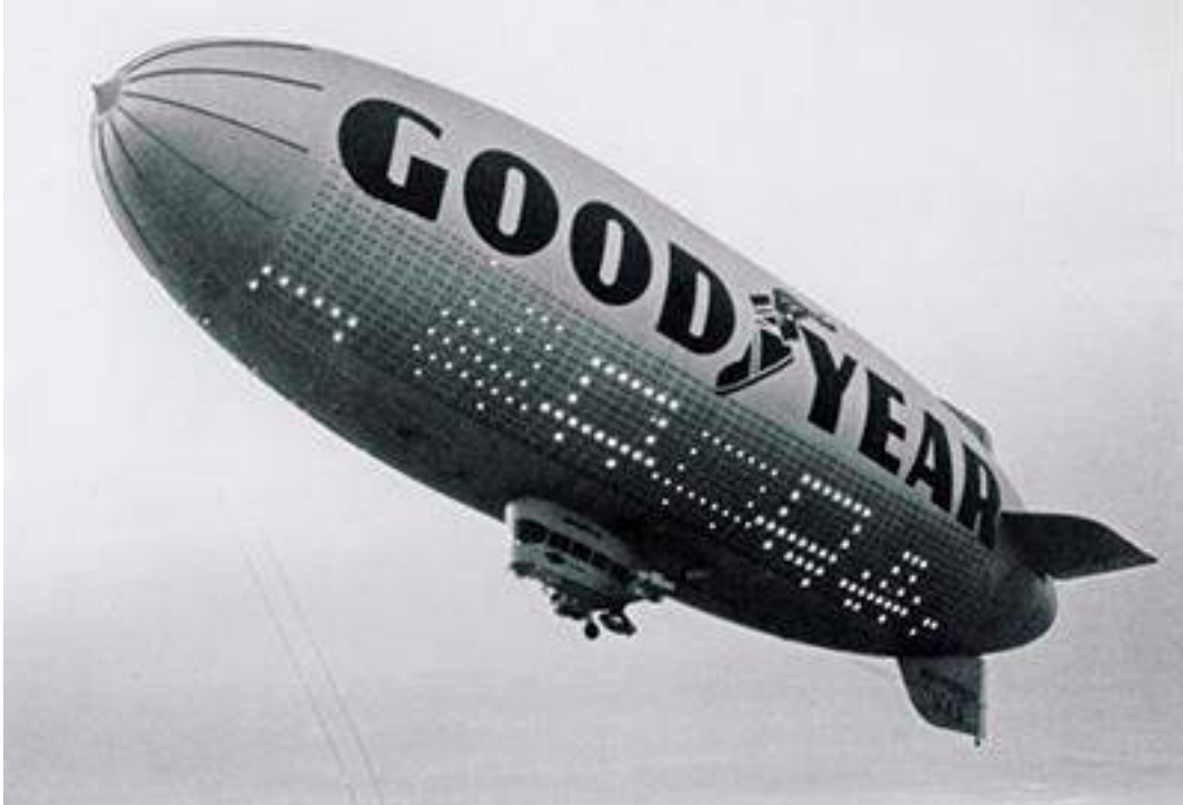
GZ-19A Mayflower introduced the “Skytacular” night sign in 1966 with 1,540 colored incandescent lights per side. Source: Goodyear
