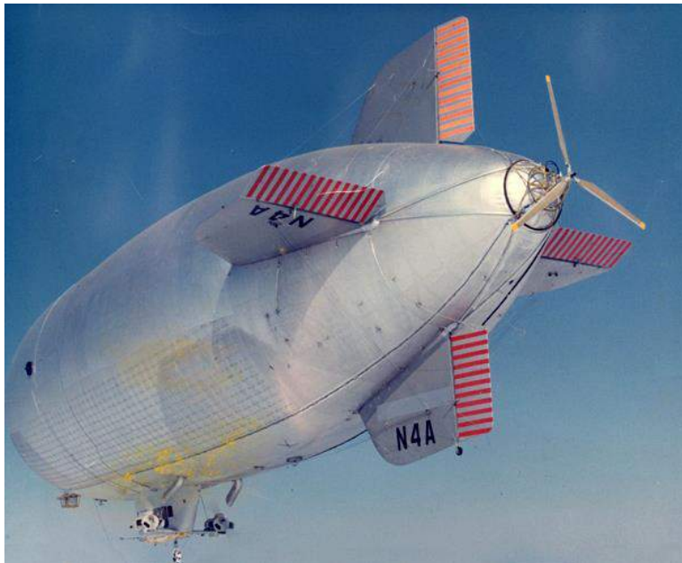
GZ-19A Mayflower with stern propeller for Silent Joe II. Source: NAA Noon Balloon, #111 (2016)
