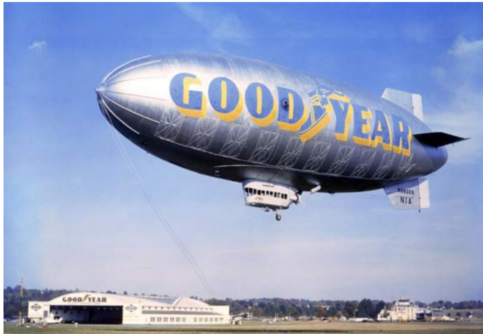
L-class Ranger with 10 Trans-Lux panels below the Goodyear logo. Source: Goodyear, circa early 1950s
