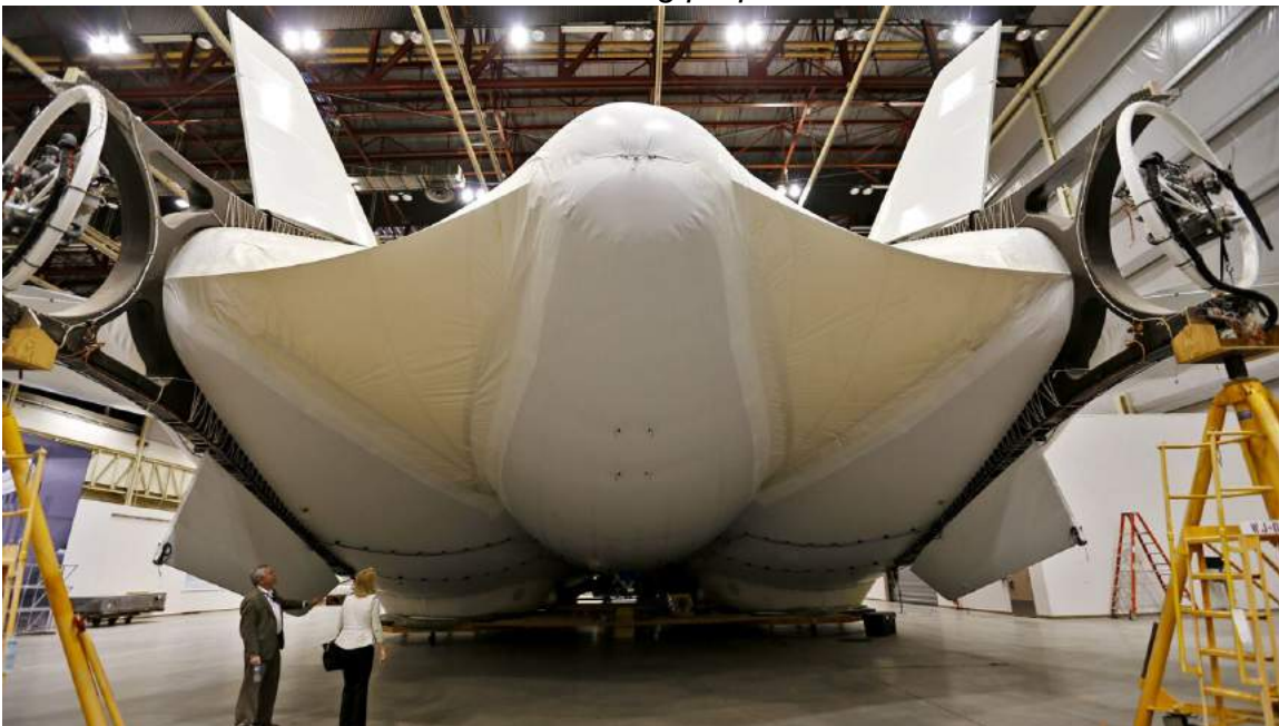
Stern view showing the two two-axis thrust vectoring propeller installations & elongated framework that distributes loads into the envelope. Source, both photos: Al Sieb / Los Angeles Times / TNS
