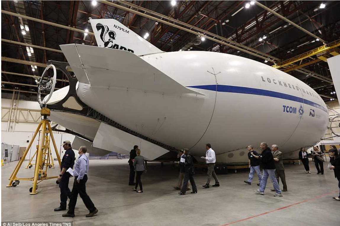
Stern quarter view showing the rear fins and one of two stern thrust vectoring propellers.
