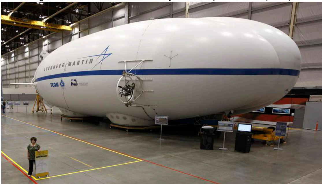
Bow quarter view showing a flank-mounted, two-axis thrust vectoring propeller. Source: Lockheed Martin
