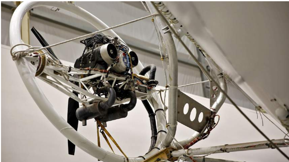
(Below) Closeup of an engine-driven, flank, thrust vectoring, three-bladed propeller installation. Source: Al Sieb / Los Angeles Times / TNS
