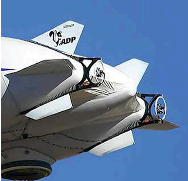
(Above left) Stern quarter view showing the aerodynamic tail surfaces and the two two-axis thrust vectoring stern propeller installations & elongated framework that distributes static & propulsion loads into the envelope. Source: Lockheed Martin
