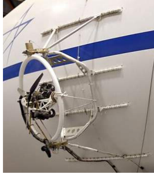
(Above left) Stern quarter view showing the aerodynamic tail surfaces and the two two-axis thrust vectoring stern propeller installations & elongated framework that distributes static & propulsion loads into the envelope. Source: Lockheed Martin
