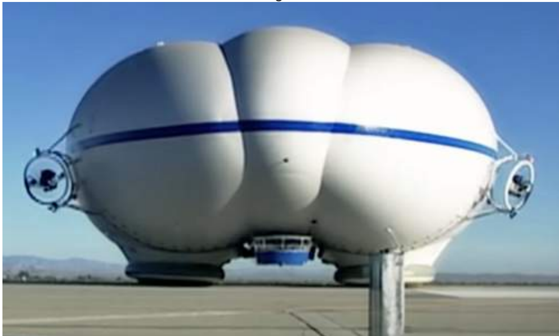
Bow view on the ground, showing the tri-lobe hull design, the gondola under the envelope's centerline, and the two forward thrust vectoring propellers. Source: Screenshot from Lockheed Martin video.
