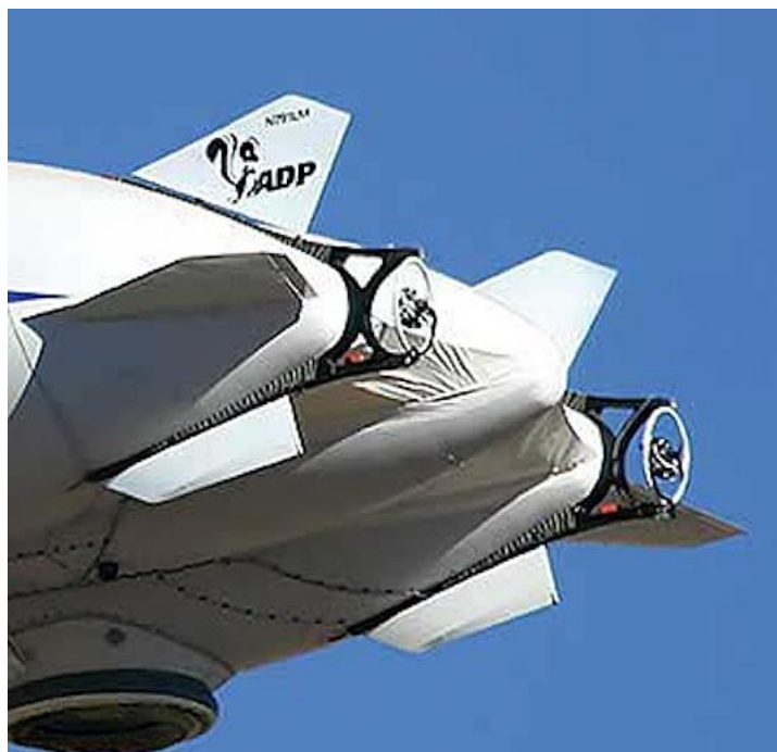
Flank vectoring thruster (left), stern vectoring thrusters (right). Source: Lockheed Martin
