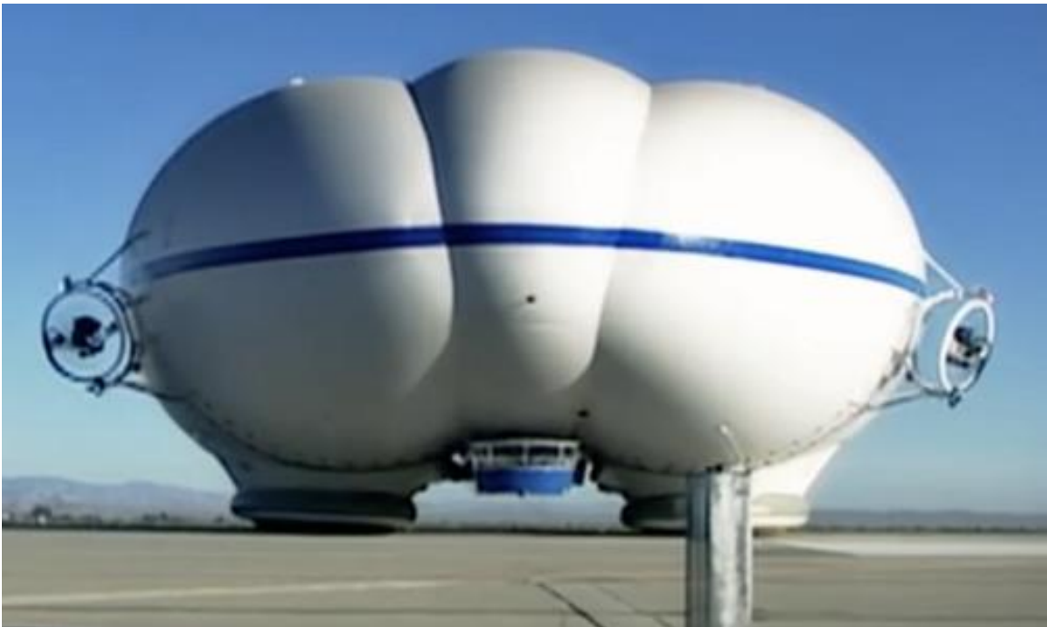
Bow view showing tri-lobe hull design and the two bow vector thrust units. Source: Screenshot from Lockheed Martin video.
