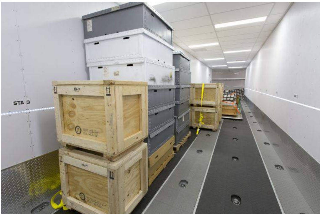
LMH-1 cargo bay contains cargo tie-downs and a strengthened deck capable of taking heavy construction vehicles and bulldozers. Source: Lockheed Martin
