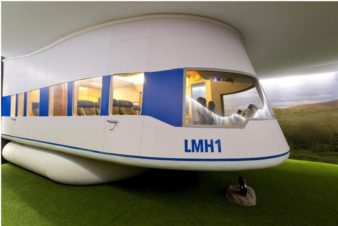
*LMH-1 gondola. Note the forward ACLS unit under the cabin.
