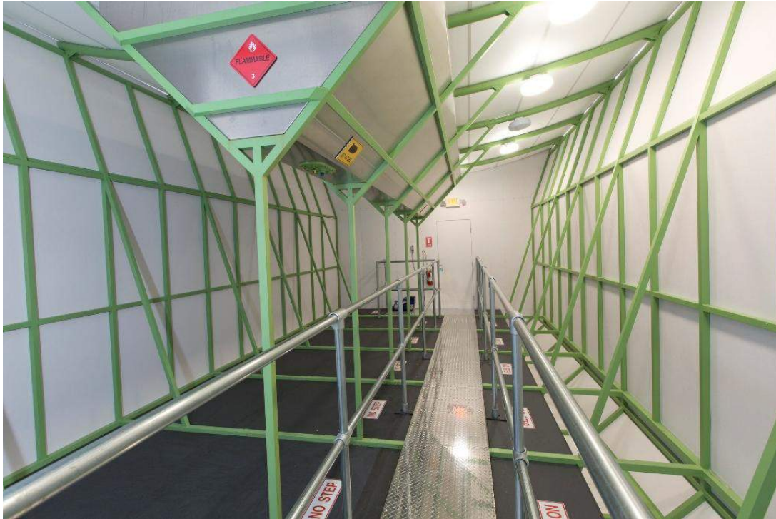
Walkway in the LMH-1 fuel bay (aka equipment bay) between the accommodation bay and the cargo bay, contains the diesel engines and associated fuel tanks. Source: Lockheed Martin
