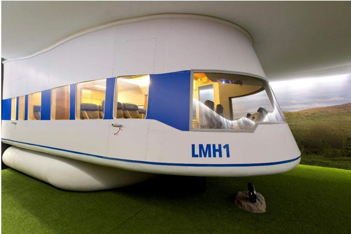
LMH-1 gondola. Note the forward ACLS unit under the cabin. Source: Lockheed Martin
