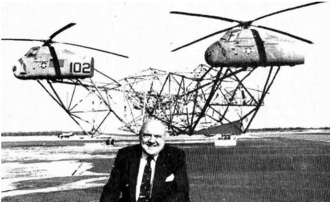
Frank Piasecki & rigid helicopter framework for PA-97-34J. Source: Flight Int'l 18 Feb 1984
