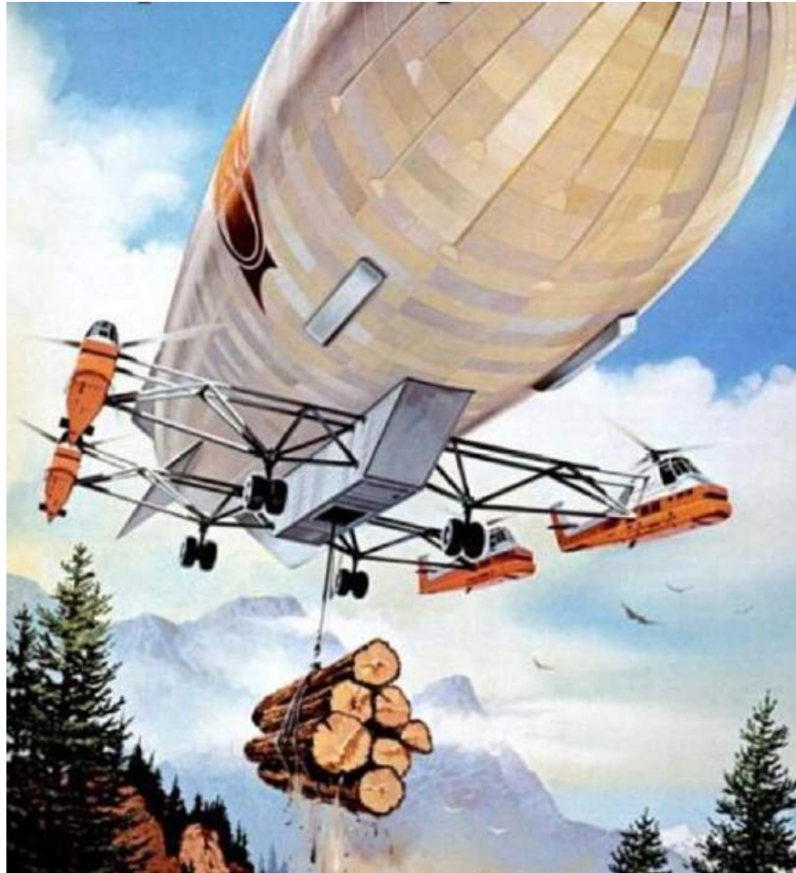
Piasecki helistat concept for the Forest Service with 4 x Sikorsky H34J helicopters. Source: Piasecki
