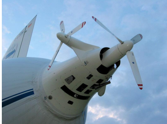
The Skybus 1500HL stern propulsor configuration (left) resembles the Zeppelin NT's vectorable longitudinal propulsor and fixed lateral thruster (right). Sources: SAIC (left), Wikiwand (right)
