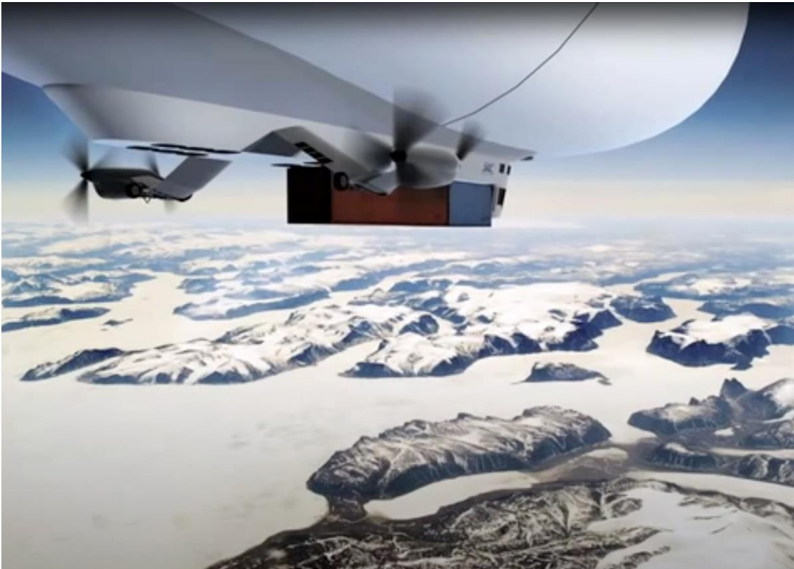
Renderings of the Skybus 1500HL flying with cargo in a remote Arctic region. Note the “push-pull” twin engine nacelles and the engine pylon configuration evident in the bottom graphic. Source: SAIC
