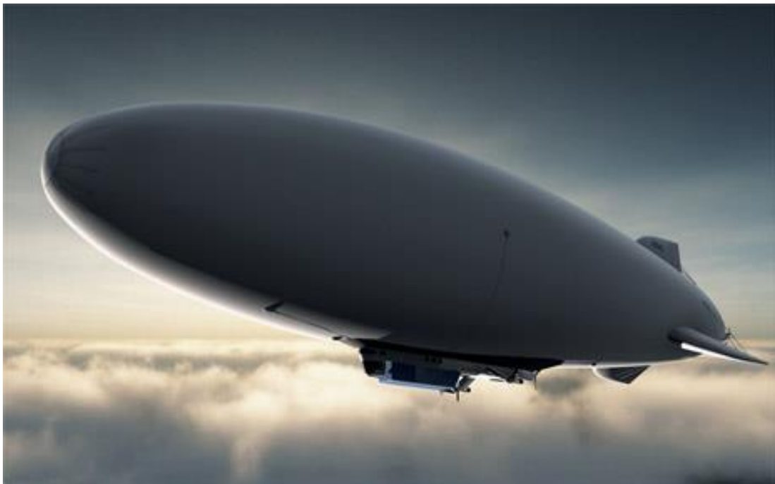
Concept drawing for an optionally manned Skybus 1500E persistent surveillance airship. Source: SAIC
