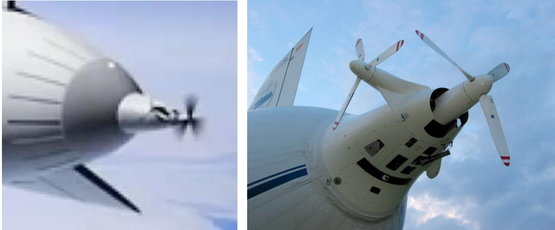
The Skybus 1500HL stern propulsor configuration (left) appears to resemble the Zeppelin NT's vectorable longitudinal propulsor and fixed lateral thruster (right). Sources: SAIC (left), Wikiwand (right)
