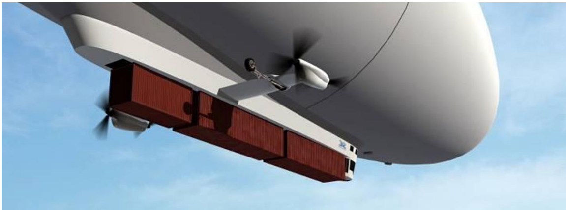
Skybus 1500HL carrying three standard CONEX boxes. Note the raised landing gear midway out on the engine pylon. Source, above & below: Melton & Hochstettler, Airships 101
