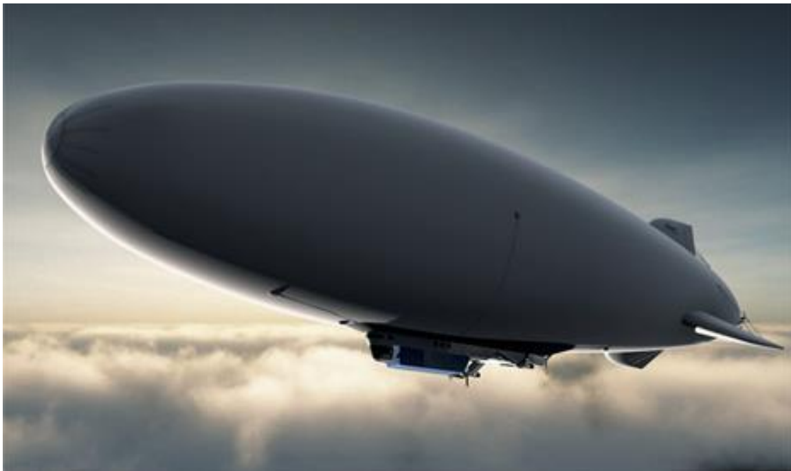
Concept drawing for an optionally manned Skybus 1500E persistent surveillance airship. Source: SAIC
