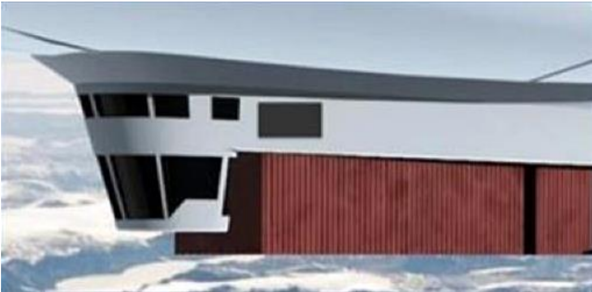
Renderings of the Skybus 1500HL carrying modular cargo containers (CONEX boxes, red) externally, secured by cargo-handling gear on the rigid keel. Source: SAIC
