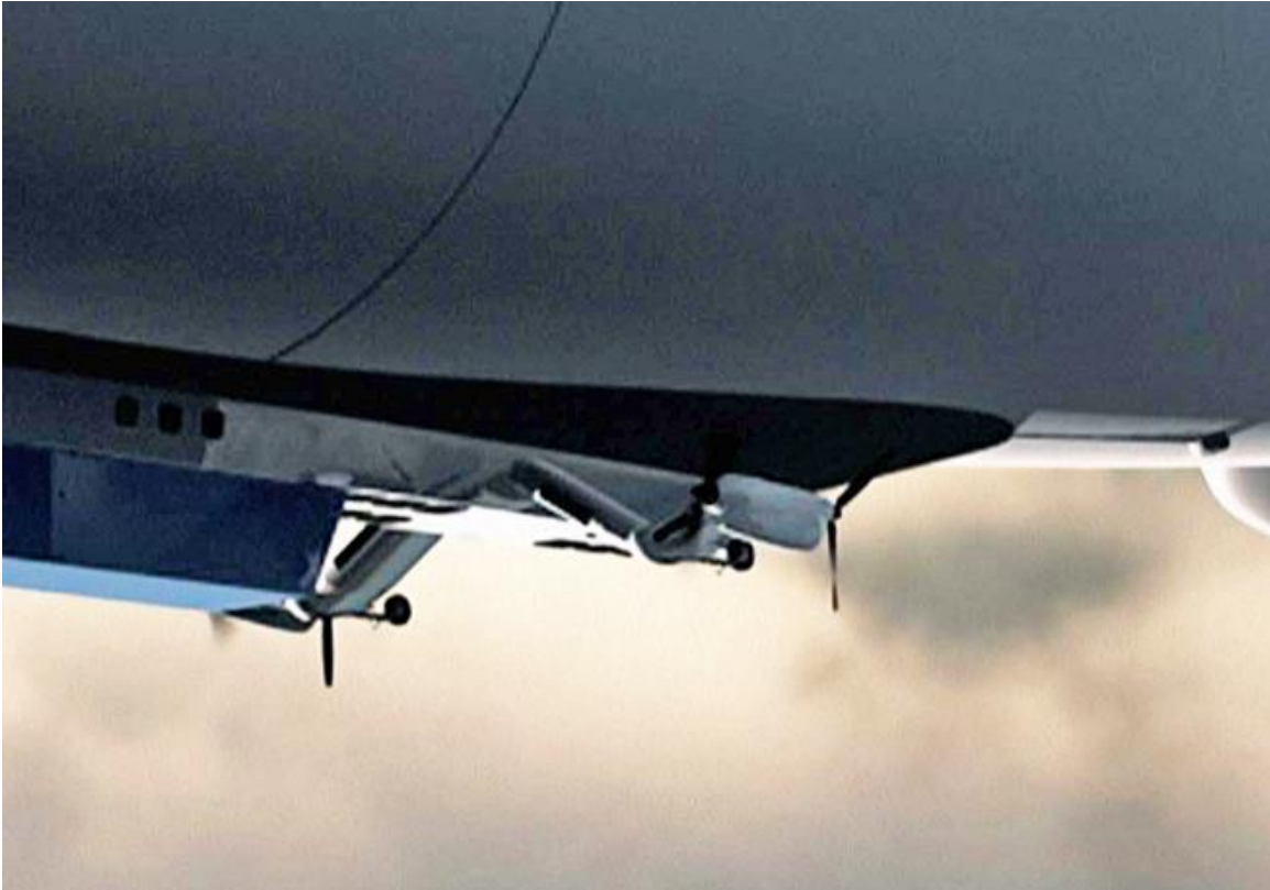
Skybus 1500E close-up view of engine layout with “push-pull” twin engine nacelles supported from the rigid keel by short pylons. Source: SAIC
