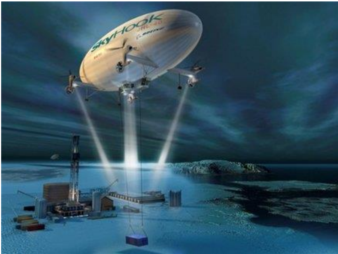
Rendering of the SkyHook JHL-40 making a load exchange. Source: Boeing / SkyHook International, circa 2008
