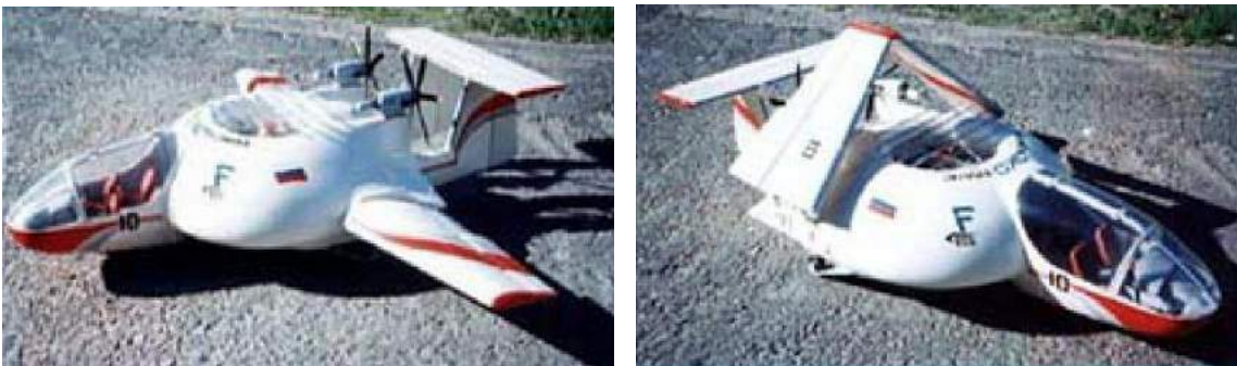
Above: Bella-1 general arrangement. Note wings folded (right). Below: Bella-1 cockpit. Source, all photos: Tumenecotrans
