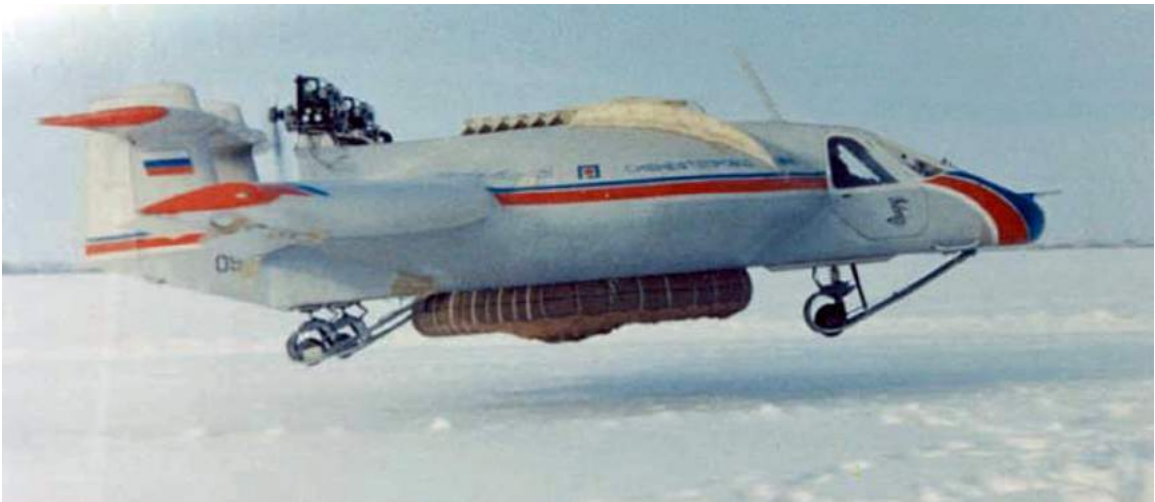
Bella-1 in flight. Note the hovercraft-style skirt under the aircraft and the skis on the tricycle landing gear to assist landing on unprepared surfaces. Source, both photos: Tumenecotrans
