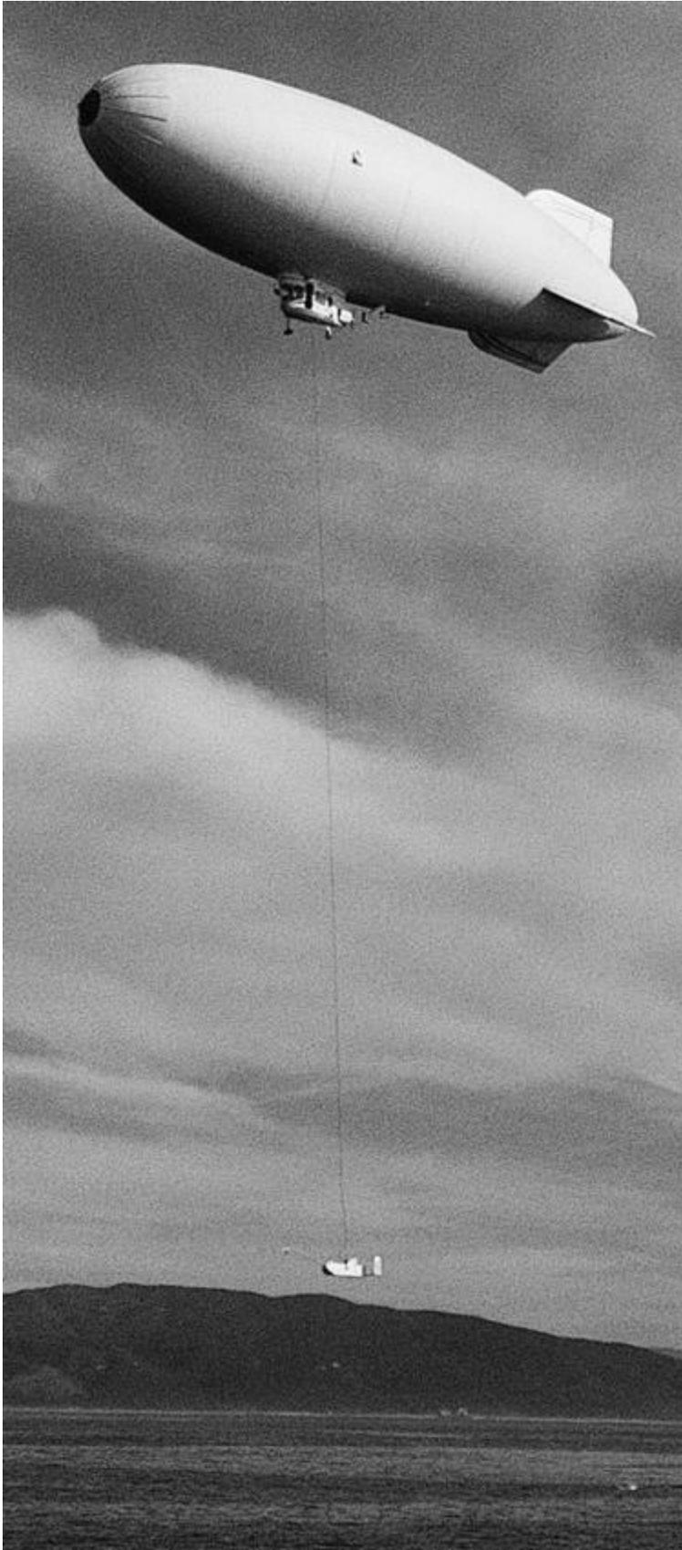
*The US-LTA Model 138S airship with the Naval Research Laboratory meteorological platform suspended 200 ft (61 m) below it to measure microwave backscatter from surface waves.
