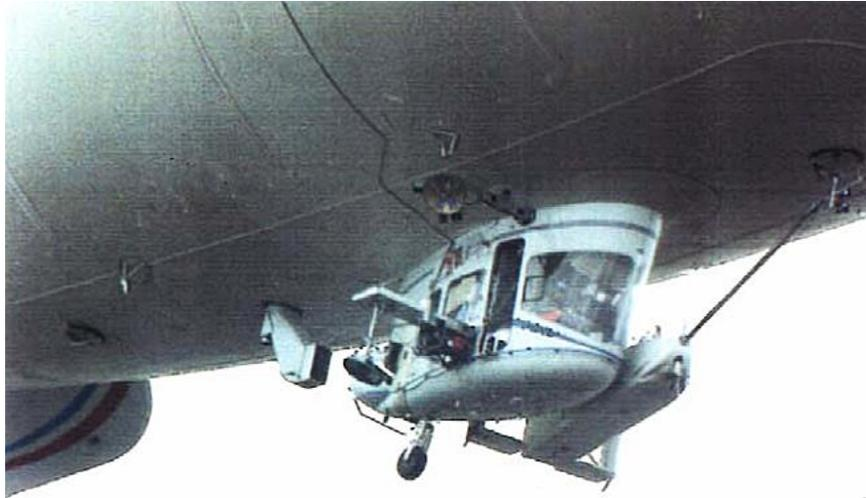
*Gondola closeup showing the configuration for an NRL project, with antennas mounted starboard side and a deployable meteorological platform stowed on the port side. Source: Eric Faure (2004)*
