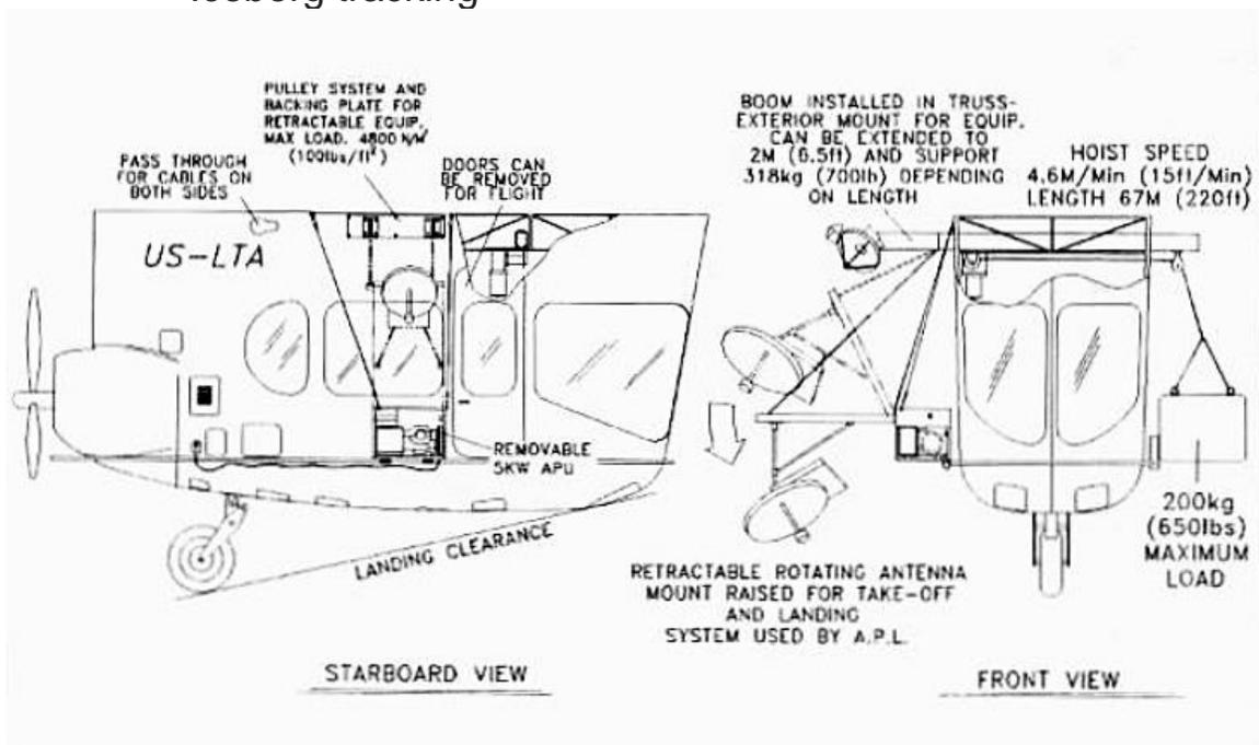
*Model 138S gondola equipped with starboard-side external sensors and port side electric hoist and deployable payload platform.
