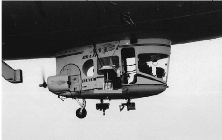
*Gondola closeup showing some of the antennas mounted for a research project. Source: D.E. Weissman (2002)*
