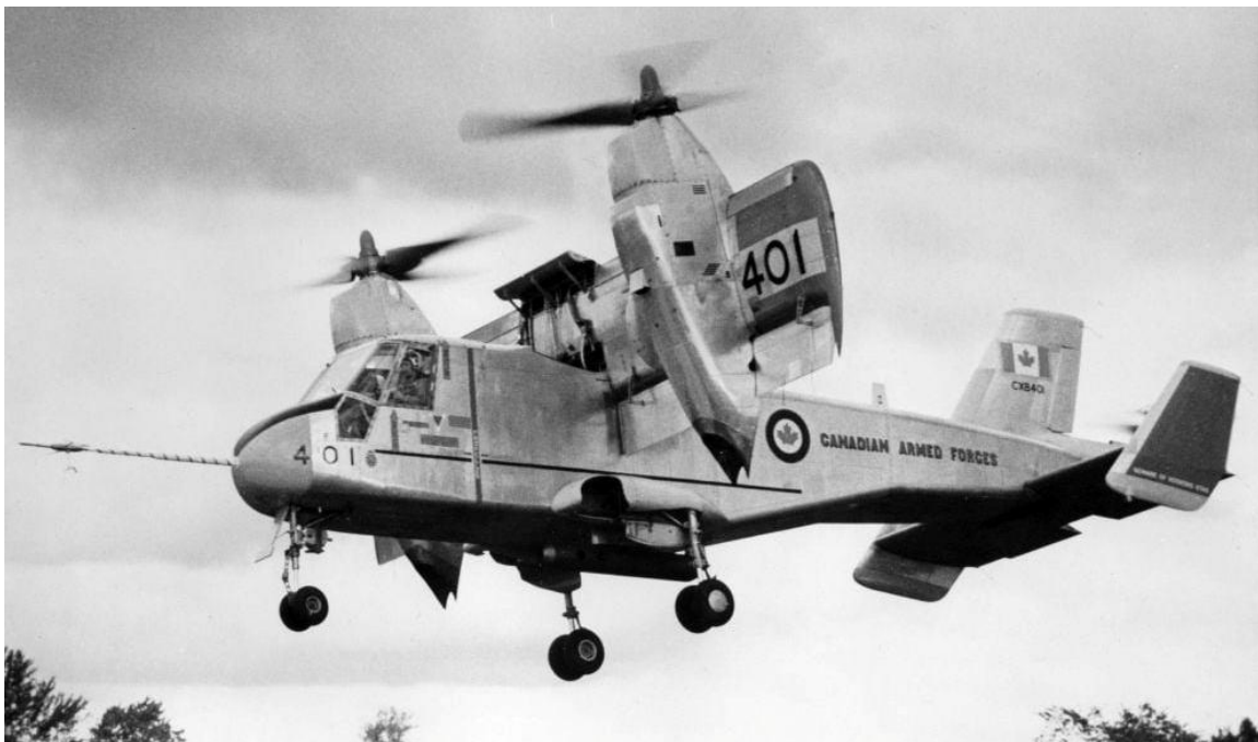
The Goodyear ZPG-X design concept used the same tilt-wing and engine configuration as the Canadair CL-84 "Dynavert" V/STOL aircraft. Source: San Diego Air & Space Museum Archives
