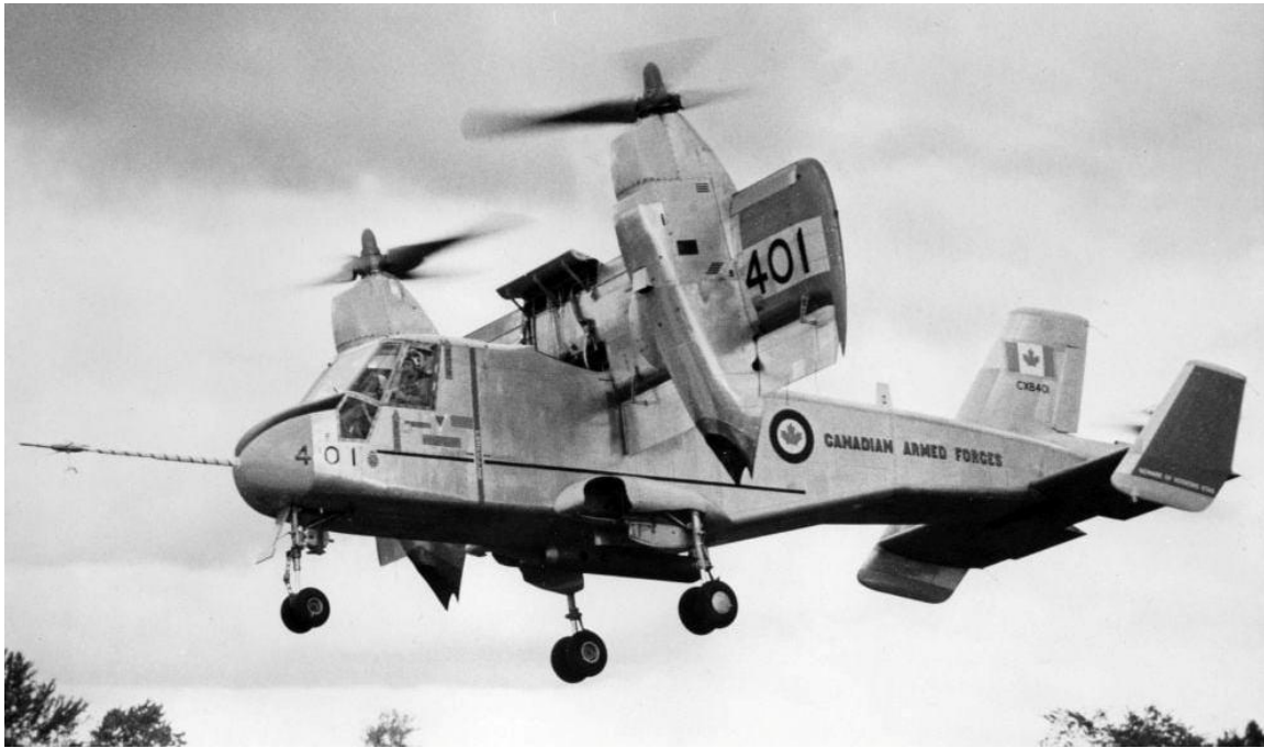
The Goodyear ZPG-X design concept used the same tilt-wing and engine configuration as the Canadair CL-84 “Dynavert” V/STOL aircraft. Source: San Diego Air & Space Museum Archives
