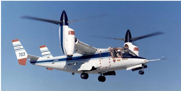
Bell XV-15 with twin Lycoming T-53 turboshaft engines that are connected by a cross-shaft and drive three-bladed, 25 ft (7.6 m) diameter rotors. Source: NASA
