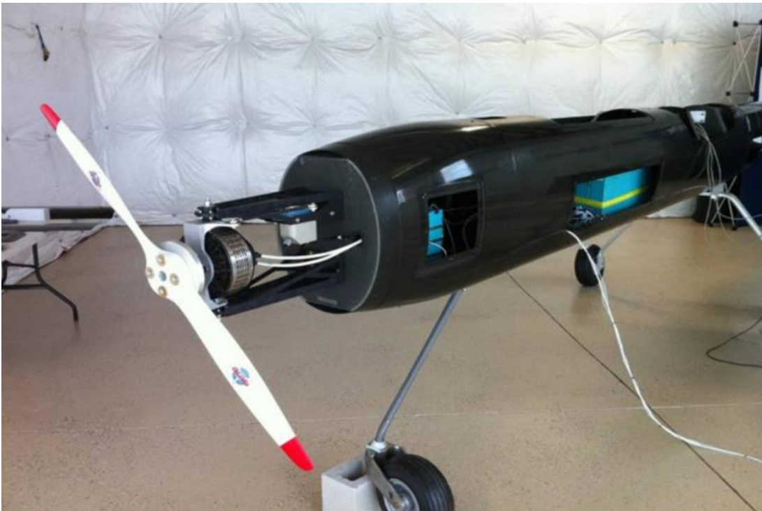
Nose propeller on the partially complete fuselage for the 40%-scale SRV demonstrator. Source: ENSS
