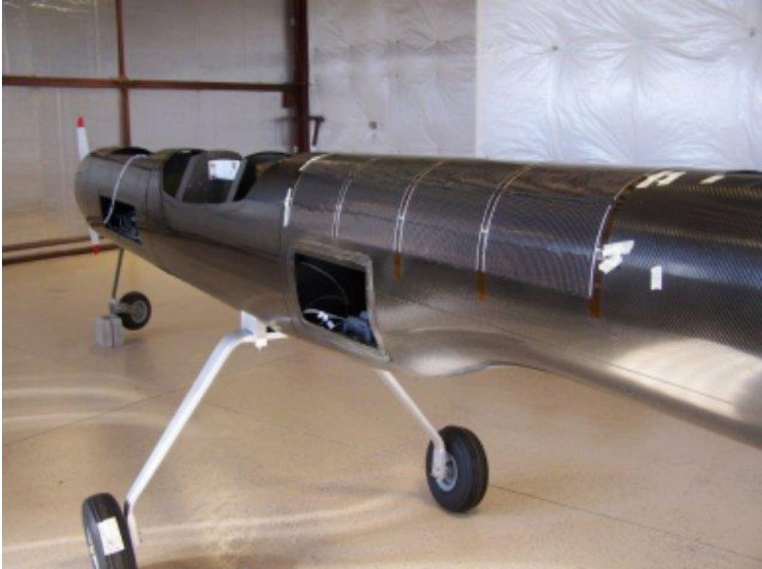
Partially complete fuselage for the 40%-scale SRV demonstrator. Source: UAS Vision
