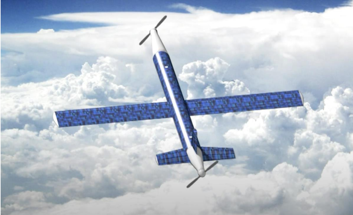
StarLight SRV with wing solar panels stowed (during ascent & fly-down).
