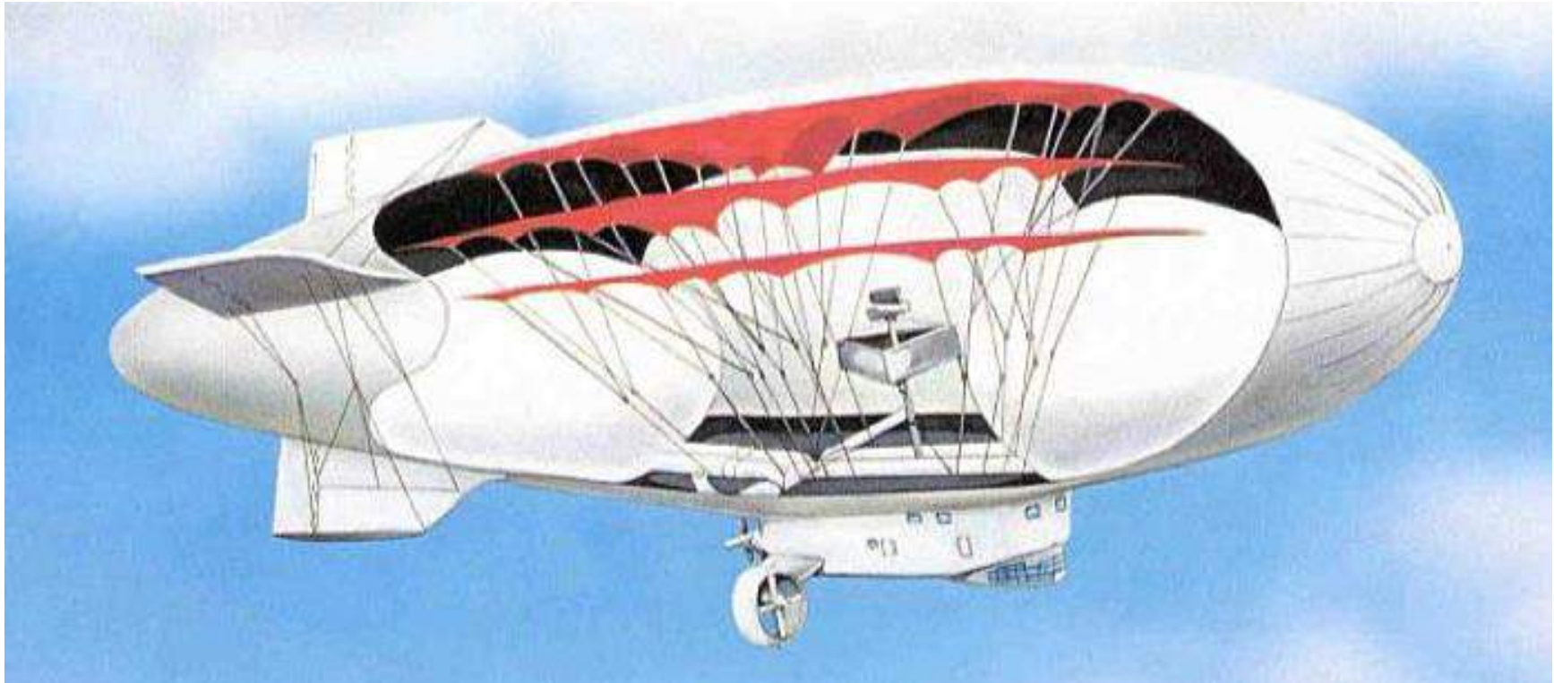
Sentinel 5000 interior details, including placement of the search radar antenna. Source: R. Hochstetler, et al., (2016)
