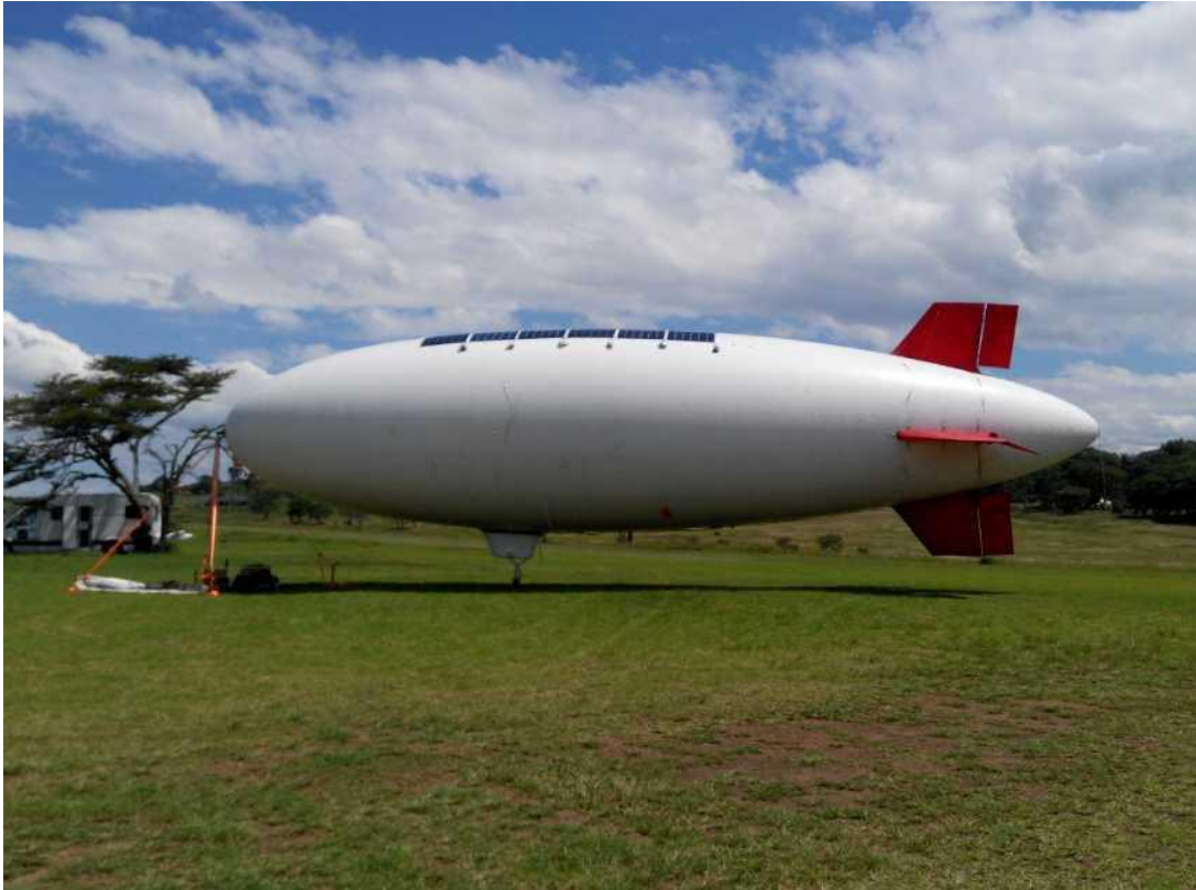
The small CA-20R solar-powered LTA drone. Source: Vantage
