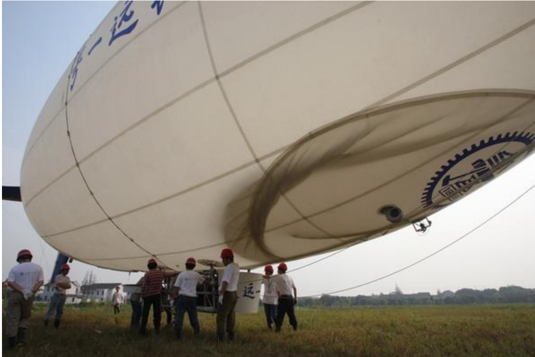
Ground handling a CA-25R LTA drone. Note the shadow of the forward ballonet on the envelope. Source: Vantage.
