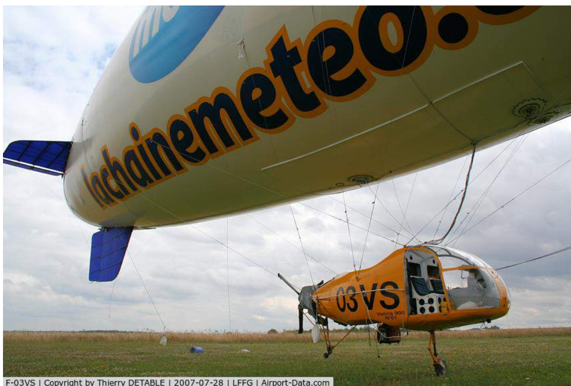
Voliris V900 two-seat suspended gondola with stern-mounted pusher propeller. Note the landing gear. Source: Thierry Detable via Airport-Data.com (28 July 2007)
