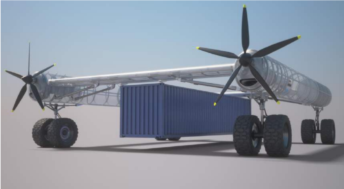
Details of the NATAC engine and landing gear nacelles and a centerline mounted standard 32T shipping container engaged by a Container Gripping Module (CGM). Source, both graphics: Screenshots from Voliris video
