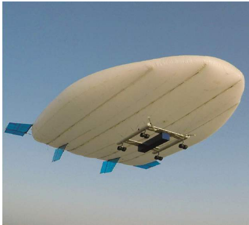
V902RC 1/7-scale Mini-NATAC demonstrator. Source: Voliris
