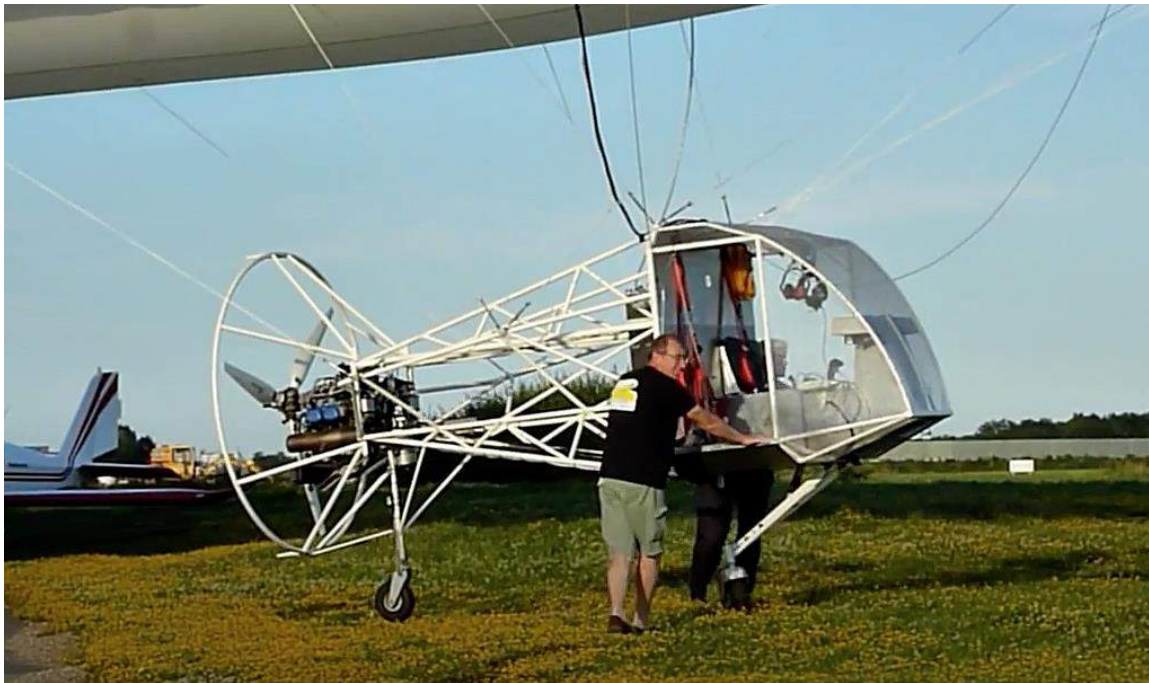
V901C suspended two-seat gondola. Source: Voliris.
