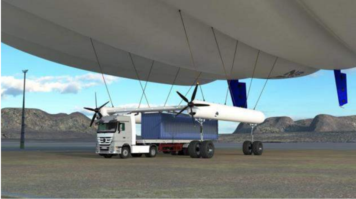
Truck unloading a standard 32T shipping container directly onto the airship's CGM. Source: Screenshot from Voliris video
