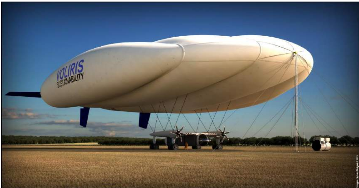
Concept drawing of an NATAC V932 hybrid airship on the ground, connected to a mooring mast. Note the suspension lines connecting the engine and landing gear nacelles to the buoyant envelope. Source: Voliris
