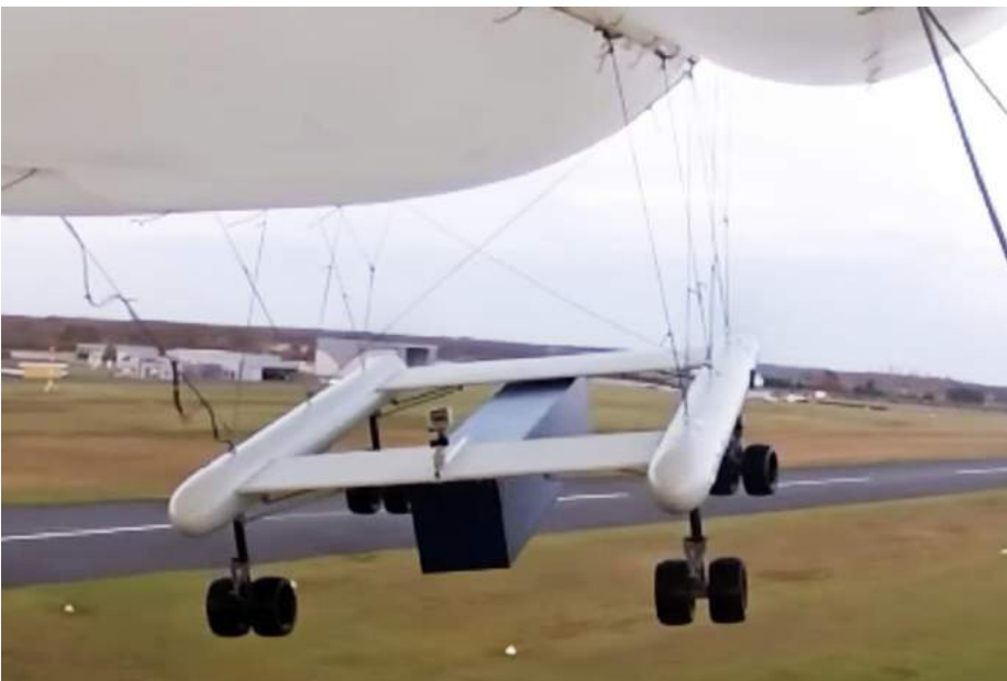
V902RC configured as the 1/7-scale Mini-NATAC demonstrator. Source, three photos: Screenshots from Voliris video
