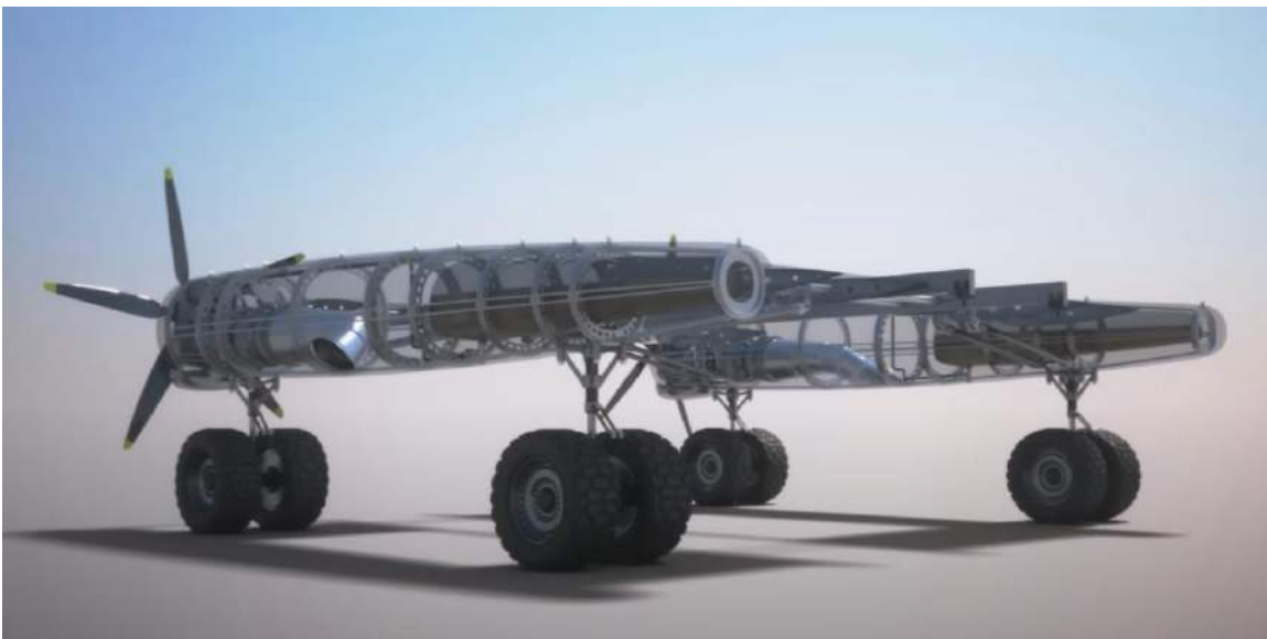
Details of the NATAC engine and landing gear nacelles and a centerline mounted standard 32T shipping container engaged by a Container Gripping Module (CGM). Source, both graphics: Screenshots from Voliris video
