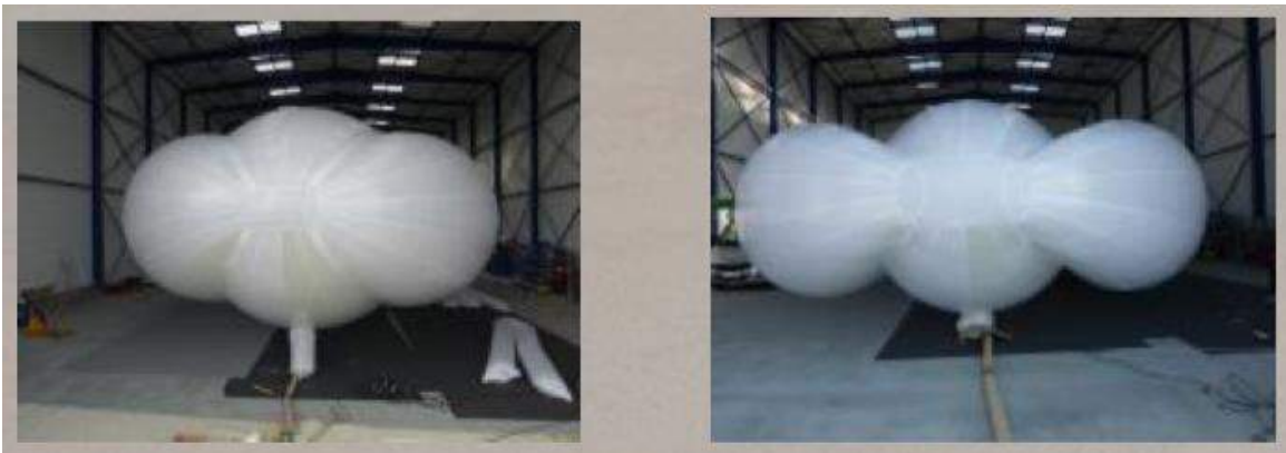
Test of the variable volume system on a tri-lobe envelope. Source: Voliris
