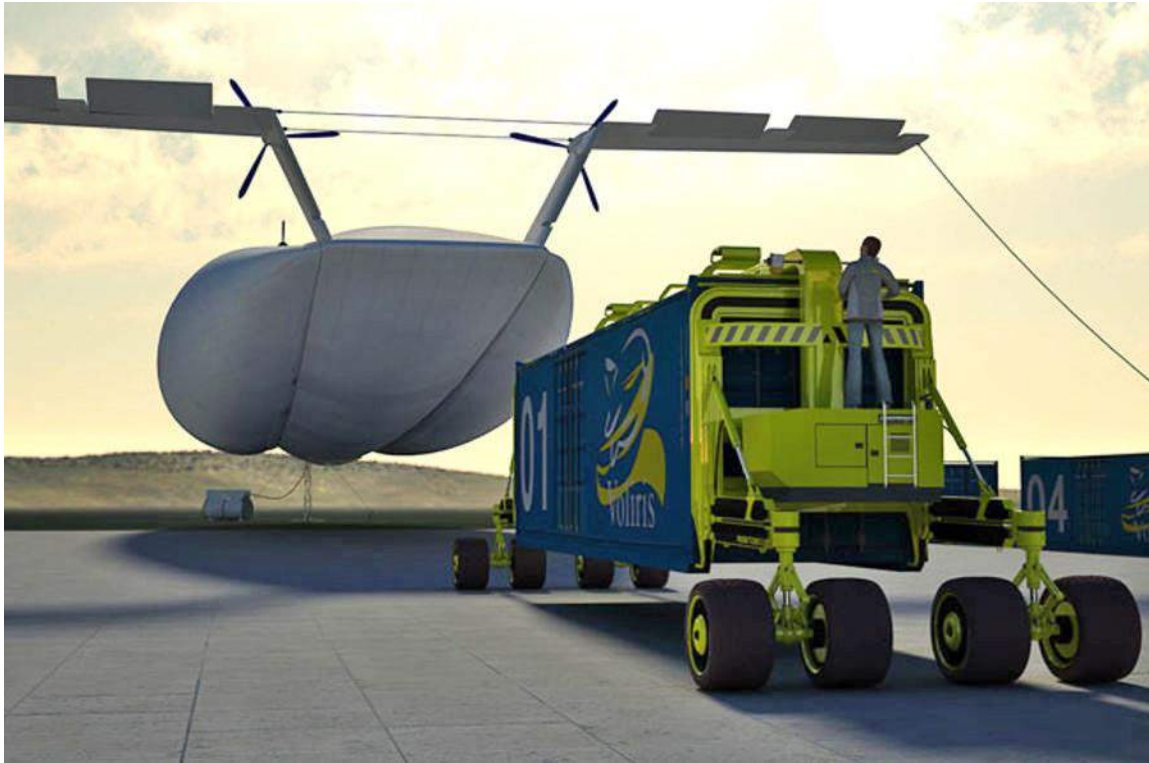
A Container Mover and Landing Gear (CMLG) unit picks up a cargo container in a freight depot and then drives under a V930 to be secured for flight.
