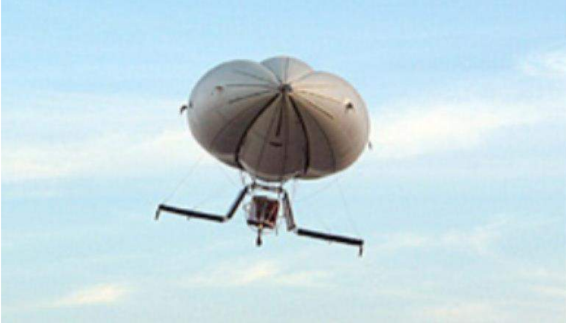
Voliris 901C head-on view highlighting the tri-lobe envelope design and the tailplane configuration. Source: Naval Airship Assoc., Noon Balloon, Winter 2012
