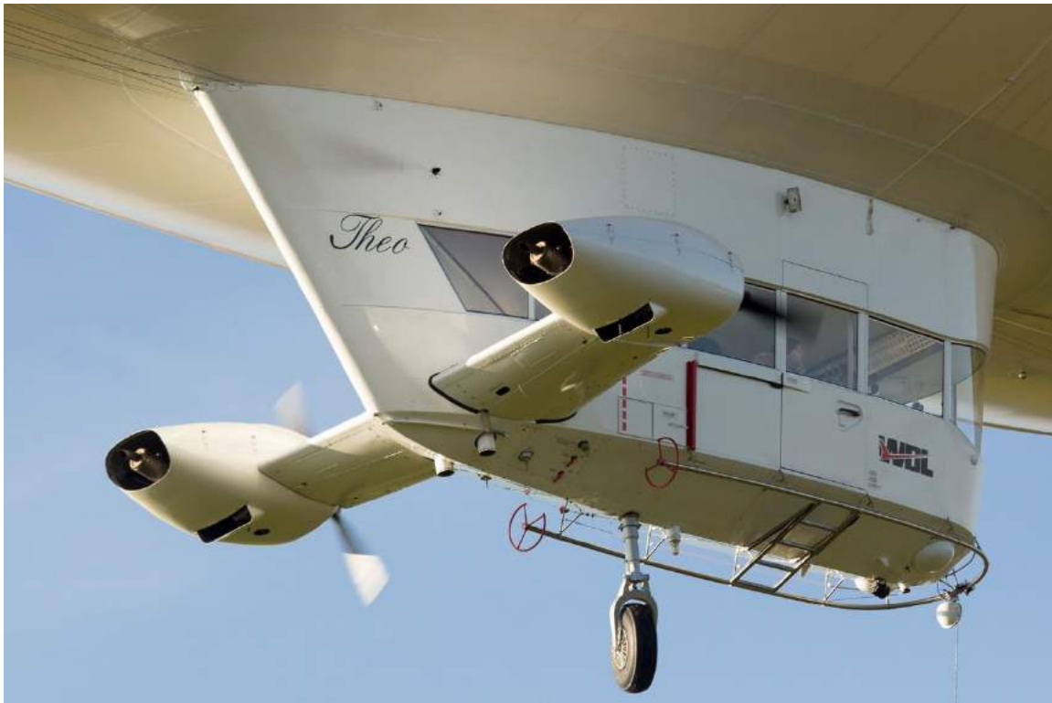
WDL-1B gondola, highlighting the installation of the Continental engines. Source: Martin, via https://www.flickr.com/photos/martinbitzer/
