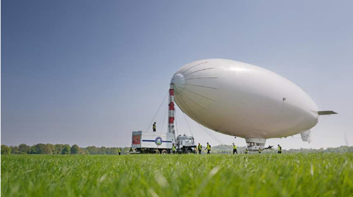
WDL-1B at a truck-mounted mobile mooring mast. Source: WDL
