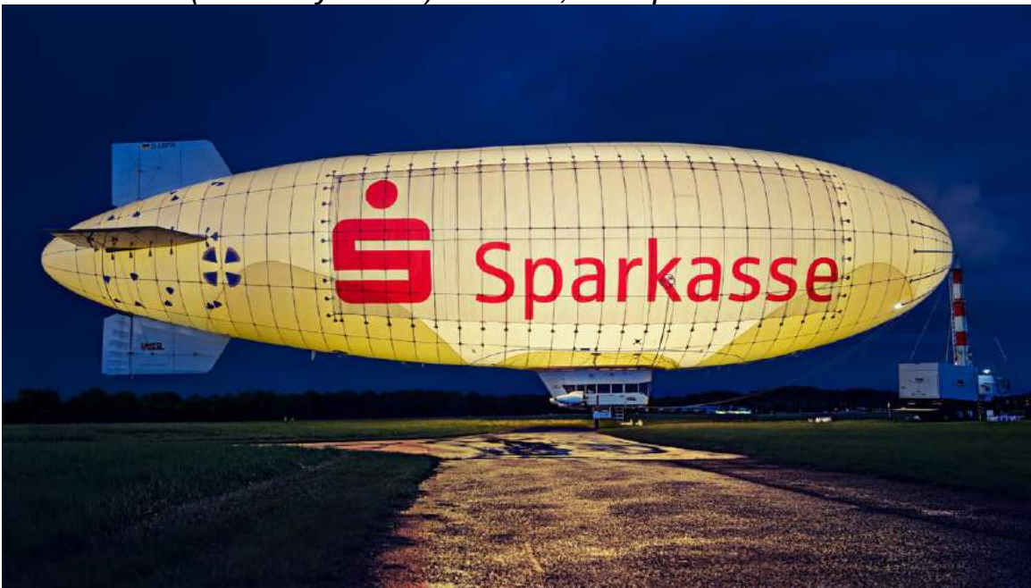
WDL-1B display system has 30 x 8 meter (98.5 x 26.2 ft) exterior hull-mounted panels (the shaded rectangle around "Sparkasse") with 9,000 lamps. Interior projectors and lighting can display animations on the translucent hull.
