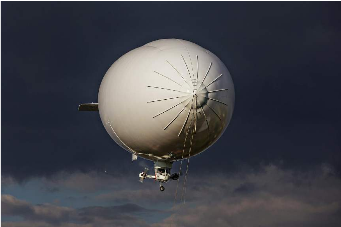
WDL-1B. Note the stiffening battens highlighted on the nose. Source: WDL
