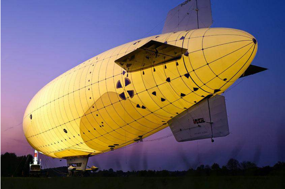
WDL-1B interior illumination highlights the internal air ballonets (shadowy areas). Source, both photos: WDL
