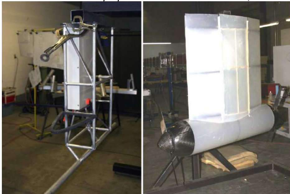
Struts attach the fixed propeller units to the equatorial structure of the airship. Source, both graphics: LTAS / Walden Aerospace
