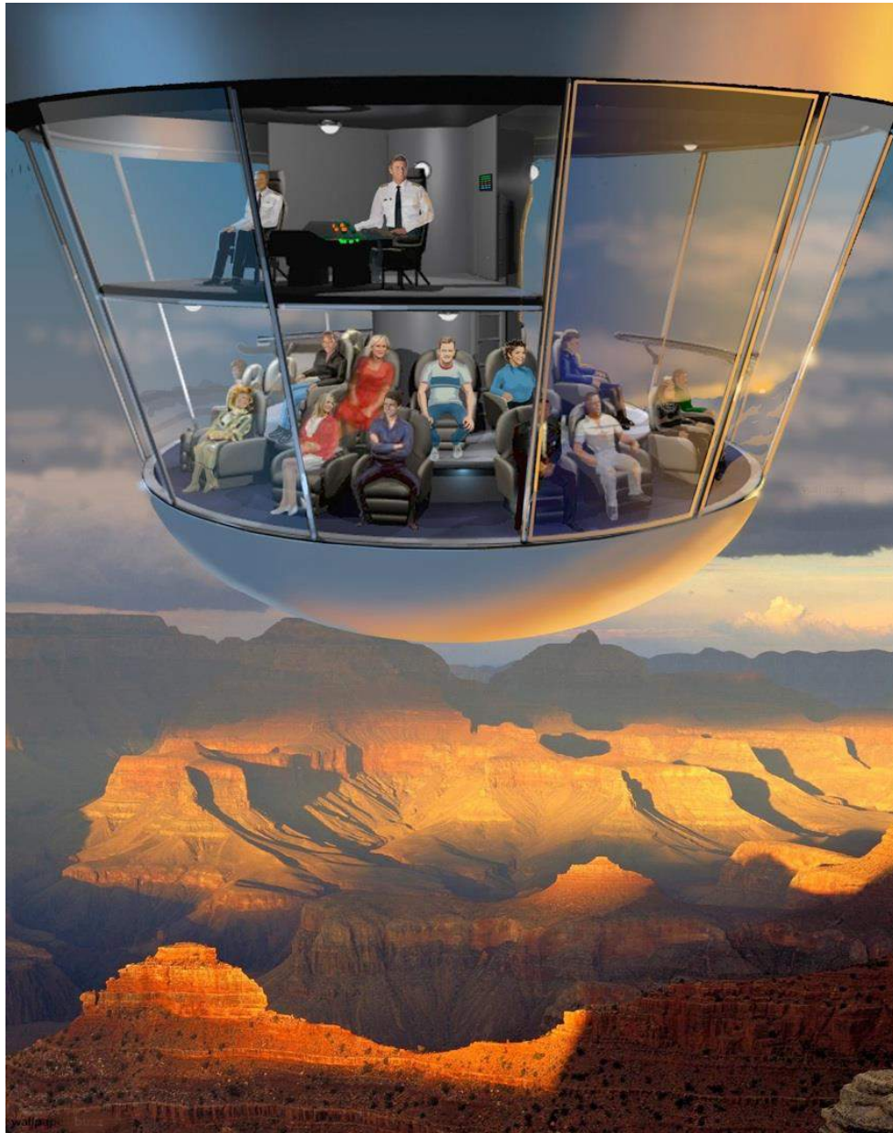
Two-level gondola configuration. Source: LTAS / Walden Aerospace
