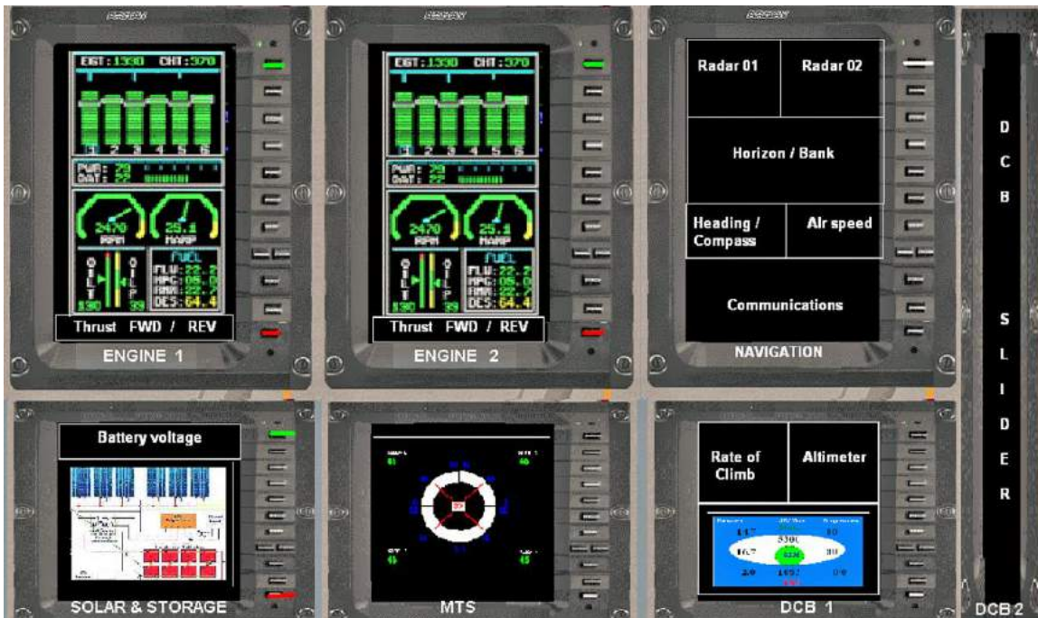
30-XB control panel in the flight simulator. Note the displays for the density controlled buoyancy (DCB) system, mass transfer system (MTS) for pitch & roll stability, and solar & battery storage system. Source, three graphics: LTAS / Walden Aerospace
