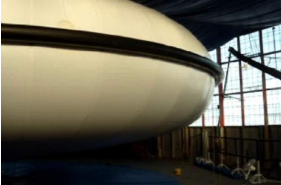
TD-2 showing the black equatorial MTU housing. Source: LTAS / Walden Aerospace (circa 2007)
