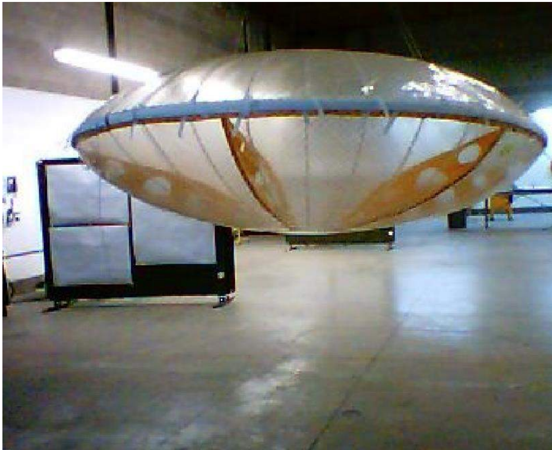
2005 pressure test flight model tethered indoors. Source: LTAS / Walden Aerospace
