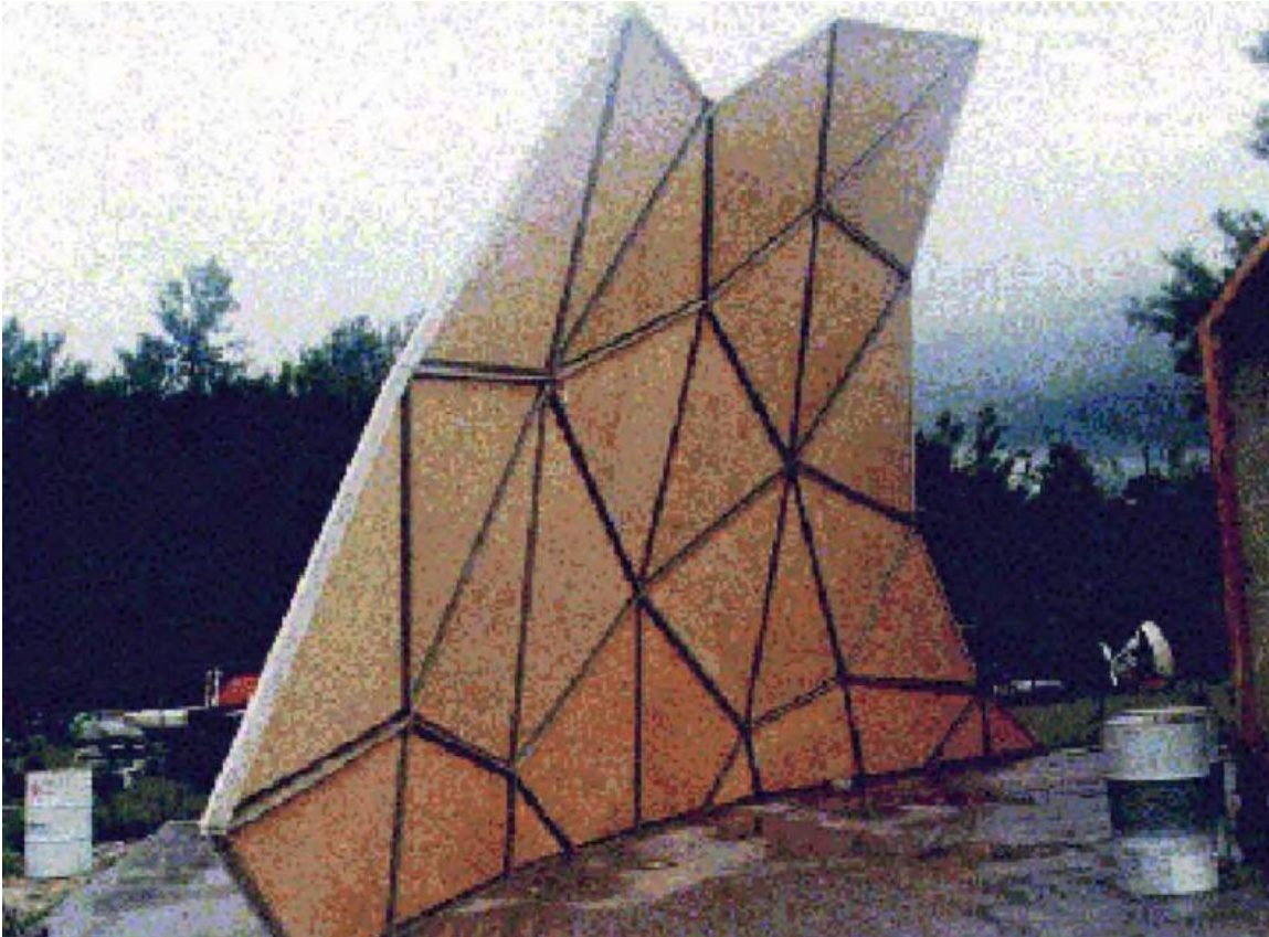
An assembled rigid, geodesic aeroshell panel. Source: LTAS / Walden Aerospace
