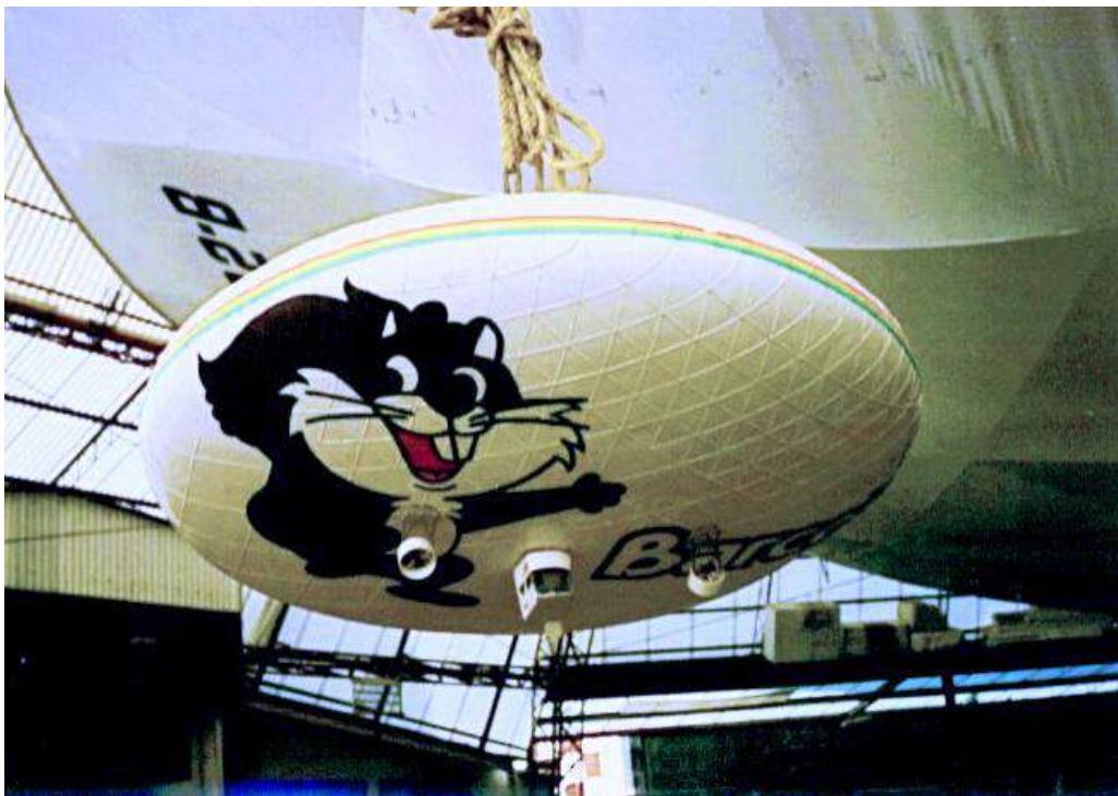
The XEM-4 subscale test model with the full-size SPACIAL MLA-32-B in the background, circa late-1980s. Note the similar triangular geodesic design of the rigid framework of the XEM-4 and MLA-32-B. Source: Walden Aerospace
