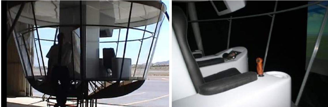
Left: Full size six-person 30-XB static test gondola, circa 2004. Right: 30-XB co-pilot station showing the side stick controller.
