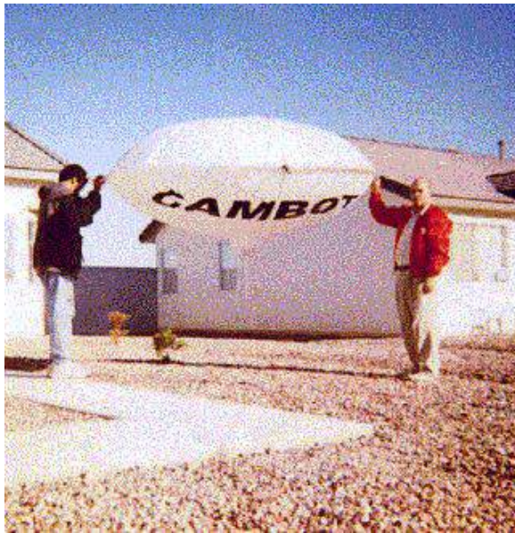
Flight of the 2.5 m (8 ft) diameter, remotely piloted, subscale CAMBOT proof-of-concept vehicle, circa 2001. Source: LTAS / Walden Aerospace
