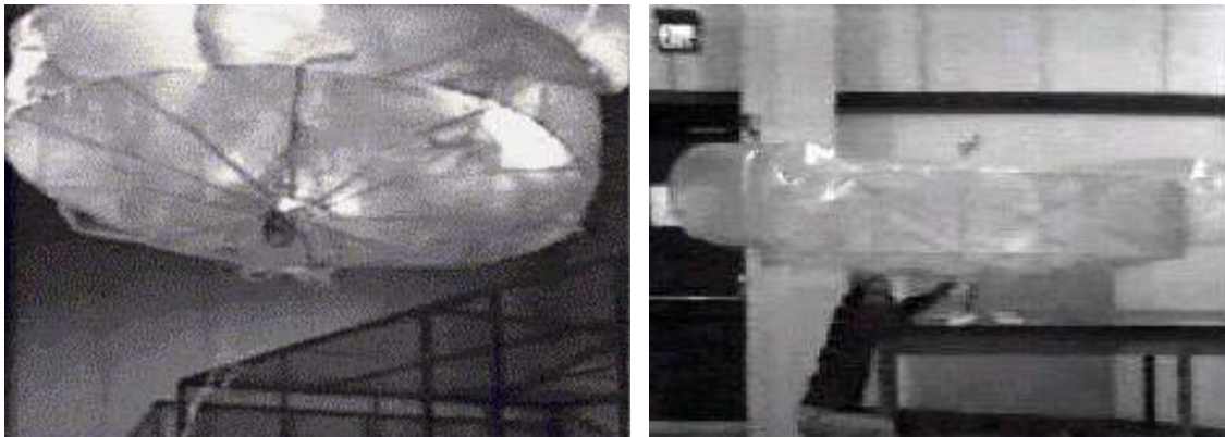
LTAS XEM-2 subscale solar powered airship showing gas cell and internal frame structure (left), which was later covered with a foam laminate rigid outer hull. Note the person under the hull (right).
