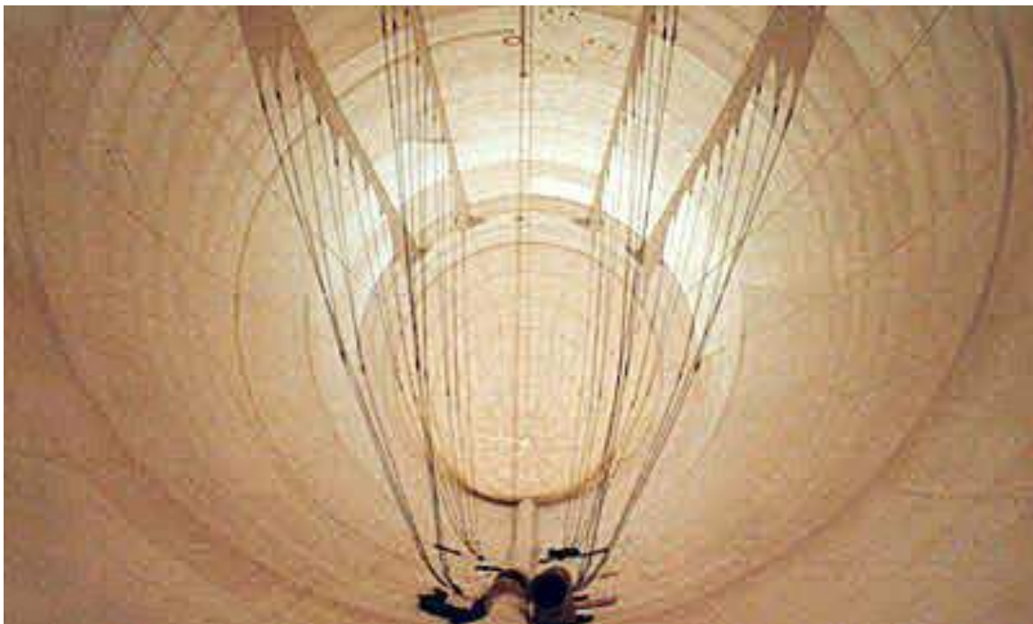
ANR-1 gondola catenary curtains inside the envelope. Source: Airship Heritage Trust
