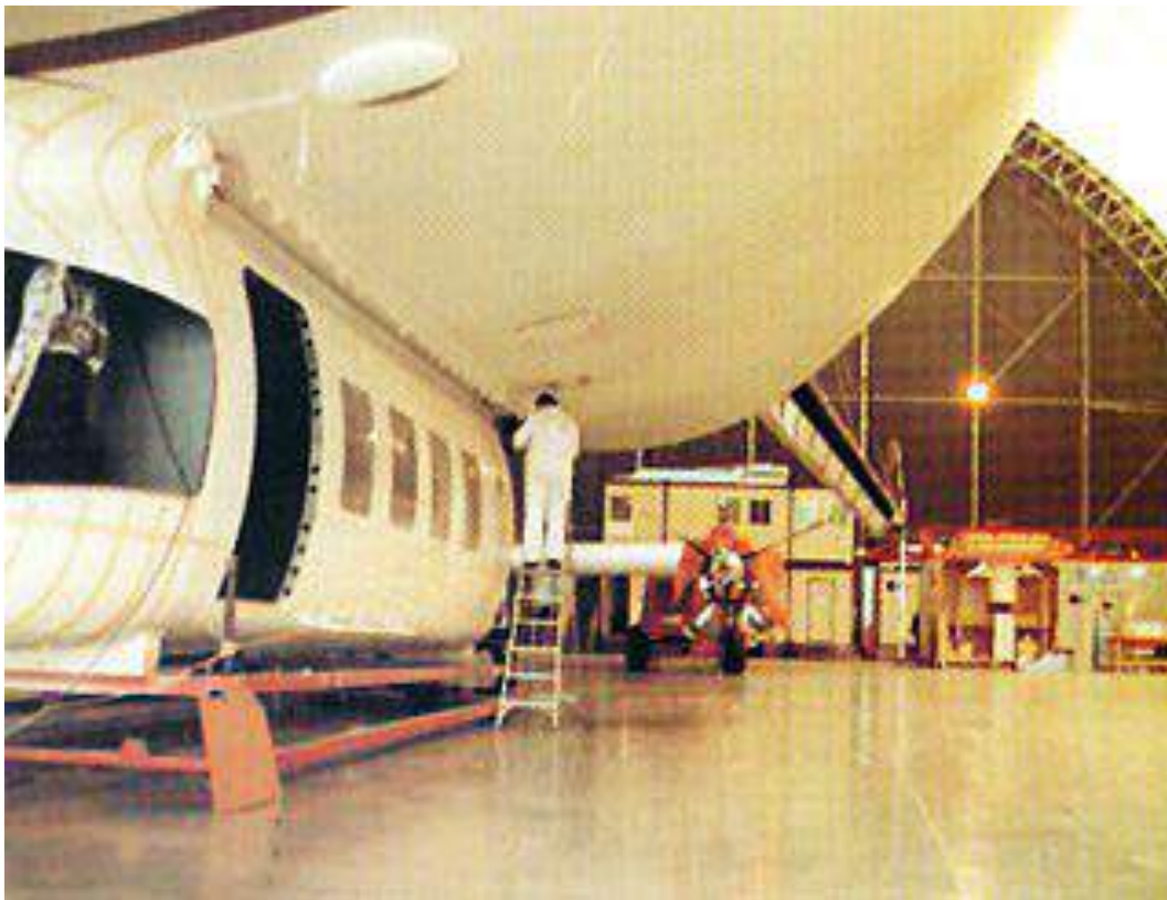
ANR-1 with gondola and fins attached to the envelope in the Jurby shed. Source: Airship Heritage Trust
