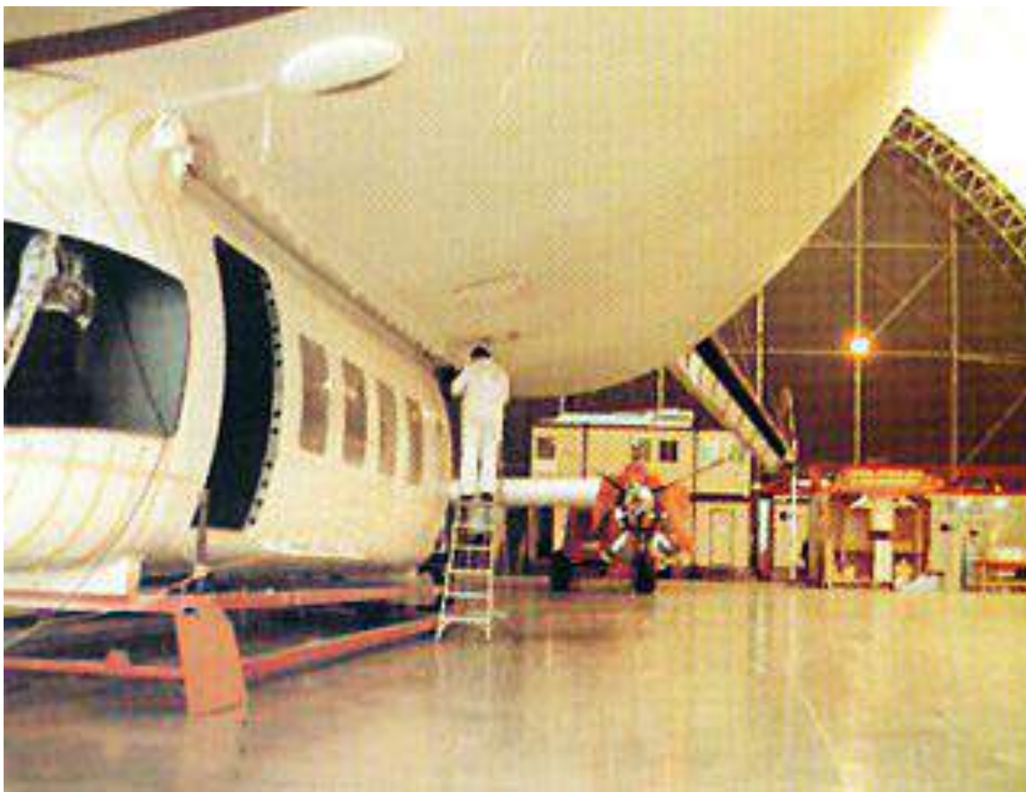
ANR-1 with gondola and fins attached to the envelope in the Jurby shed. Source: Airship Heritage Trust
