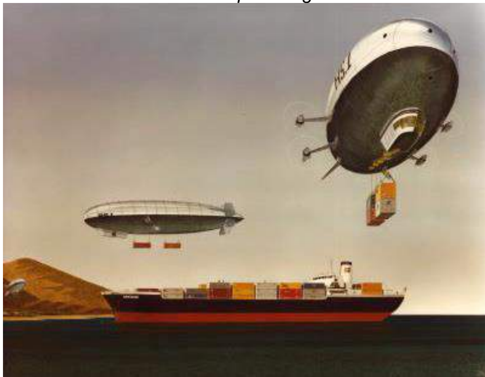
RS.1 offloading a ship. Note the four turboprop main engines mounted on stub wings. Source: Airship Heritage Trust
