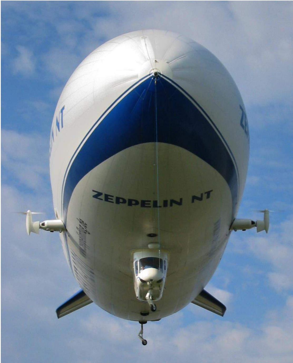
Bow view showing the flank thrusters vectored up for takeoff or landing. Source: Hansueli Krapf via Wikipedia
