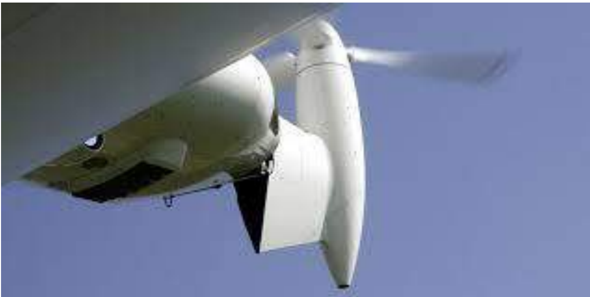
Flank thruster in the "full up" position. It can be vectored between 90° up and 30° down.
