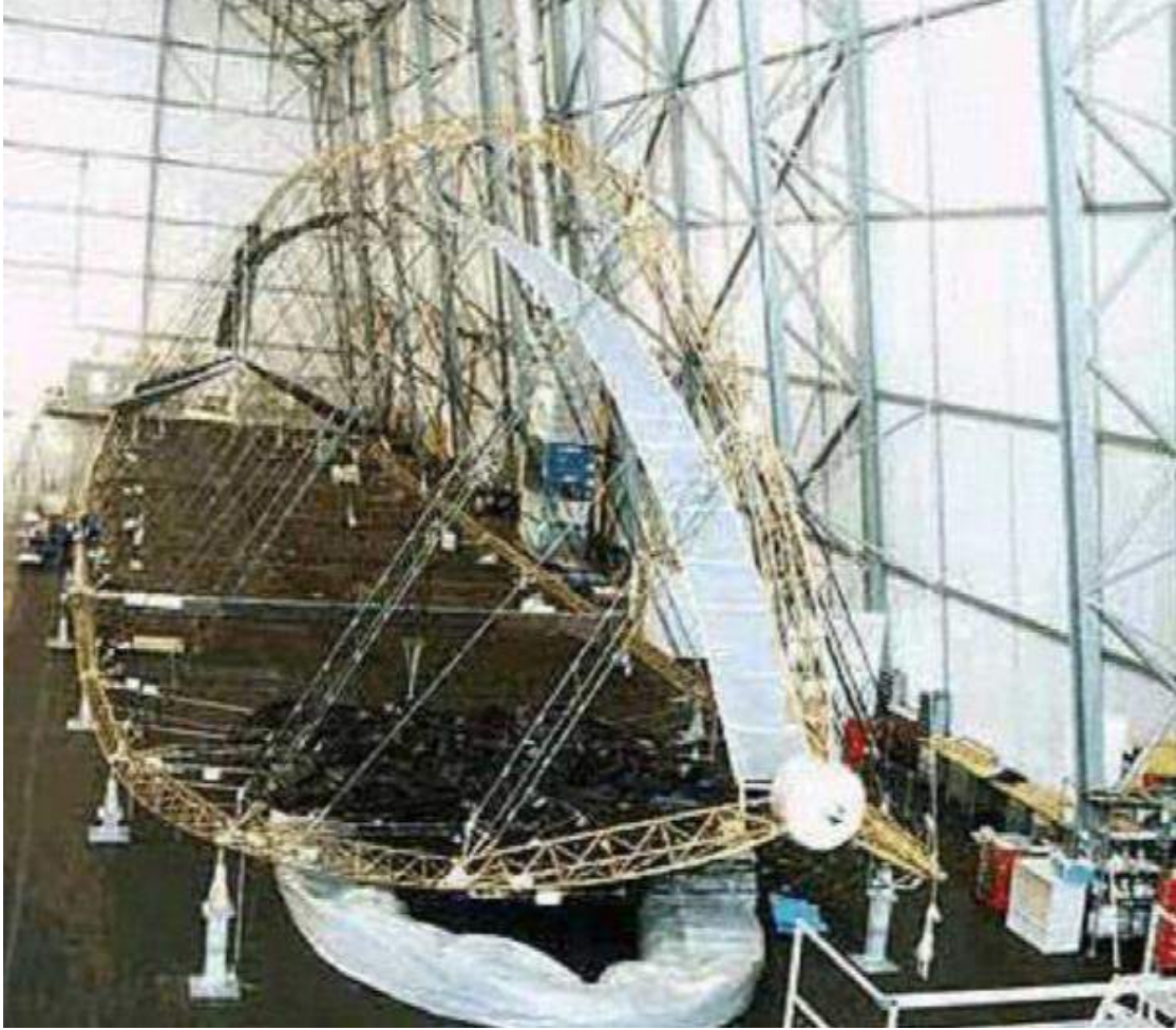
Installing the flexible fabric envelope over the Zeppelin NT's rigid internal structure. Source: Screenshots from video, ZLT Zeppelin Luftschifftechnik GmbH
