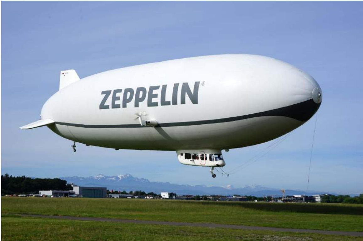
On approach to landing, with flank thrusters in the vertical position for lift. Source: Author's photo
