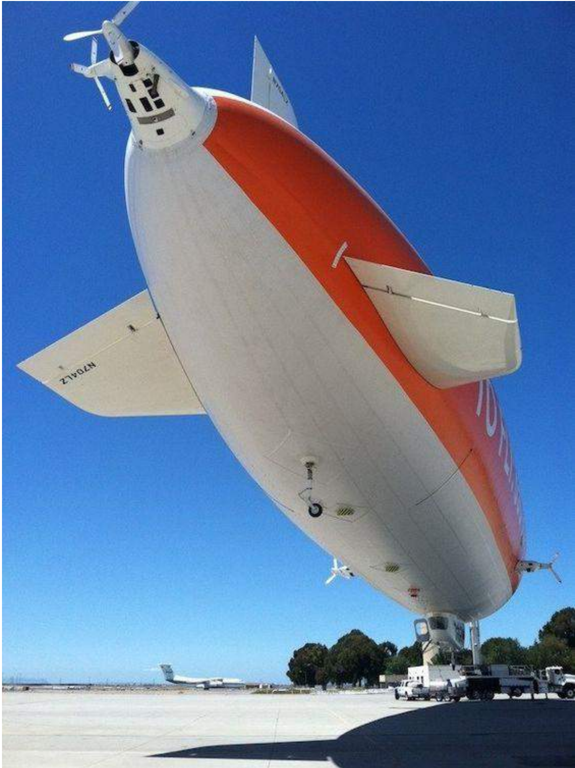
Zeppelin NT Eureka stern thrusters: one fixed lateral thruster and the main propulsion thruster that can be vectored 90° down.
