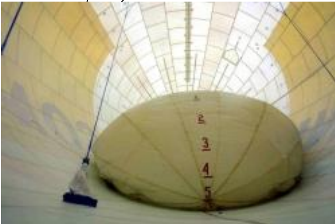
Inside the Sky Dragon envelope, looking forward from above the gondola. Note the catenary cables carrying the weight of the gondola into the upper surface of the envelope. Above: deflated forward ballonet. Below: partially inflated forward ballonet. Source: Aeros
