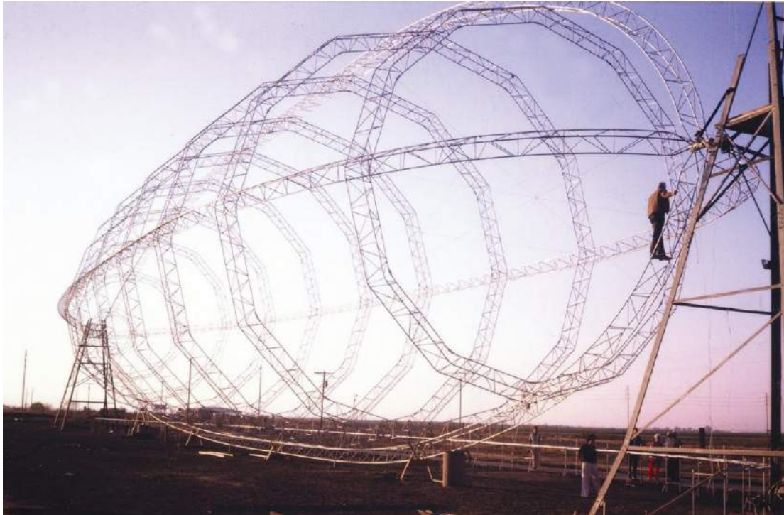
The Conrad CA220 dirigible hull early in construction. Source: Darwin Conrad via MakeHigleyHistoric
