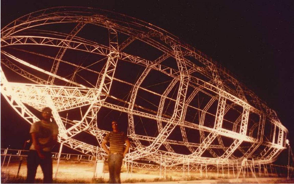
The Conrad CA220 dirigible hull under construction at night. Source: Darwin Conrad via MakeHigleyHistoric
