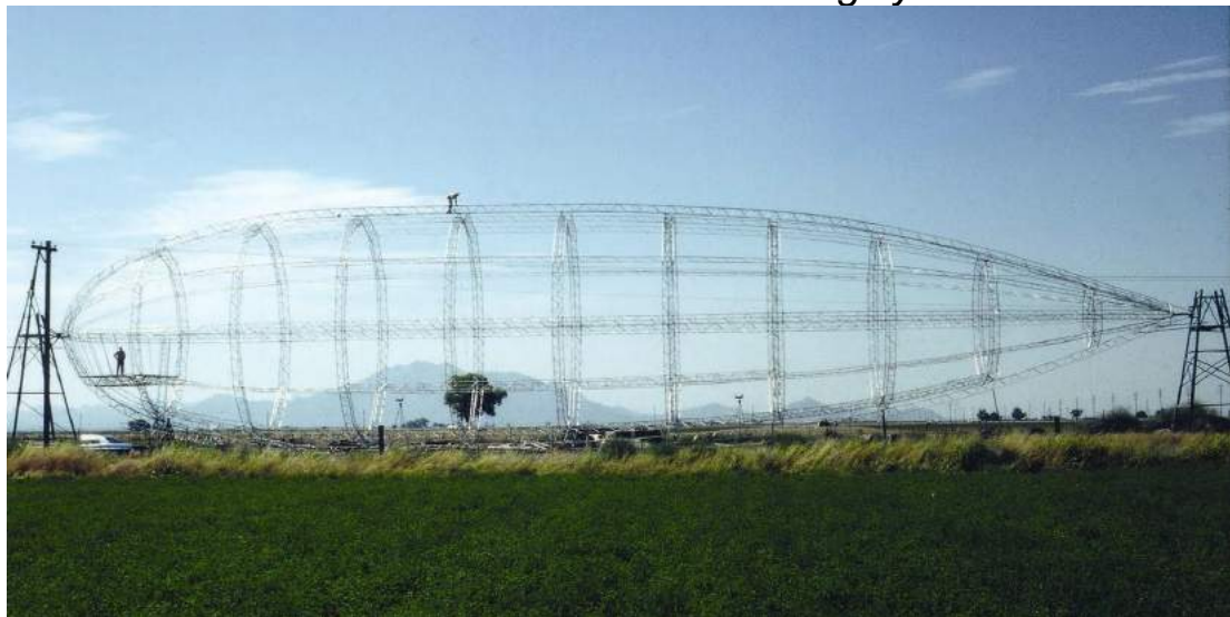
The Conrad CA220 dirigible, profile view of the rigid hull during construction. Source: Darwin Conrad via MakeHigleyHistoric
