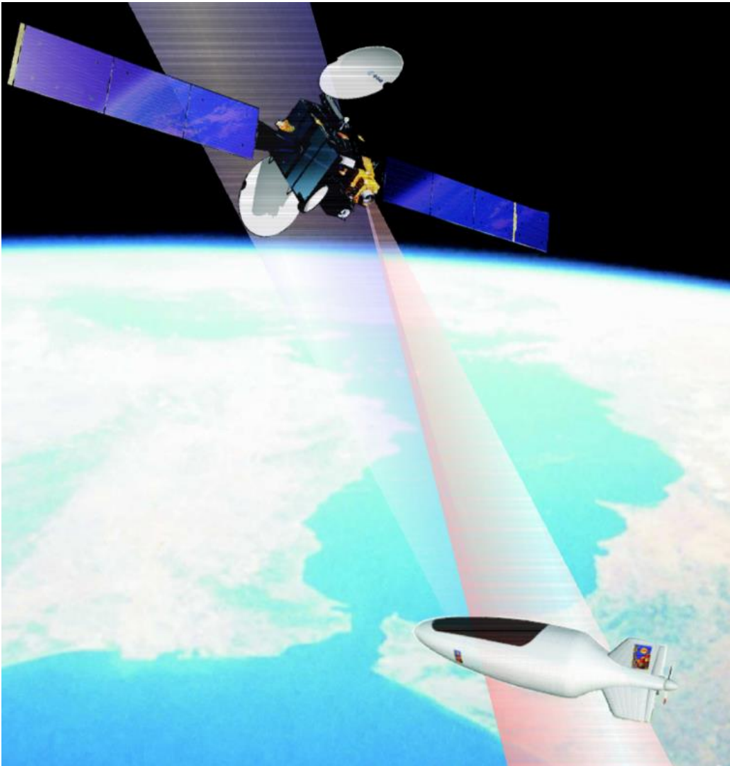
Free space optical communications links between an ESA / Lindstrand HALE stratospheric airship and an orbiting communications satellite. Source: F. Fidler, Dissertation (2007)
