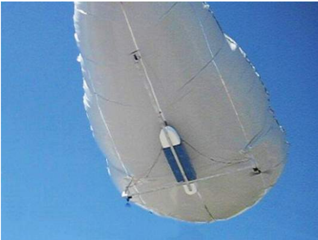
1:20 HSSA model carrying a scale model cargo container. Source, both photos: Inhabit (2010)
