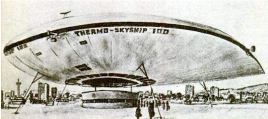
A Thermo-Skyship sits on long retractable landing legs with the payload module lowered to the ground. Note the steep passenger boarding ramp in the graphic below. Source: LTA Solutions (above), Thermo-Skyship Ltd. 1979 proposal (below)
