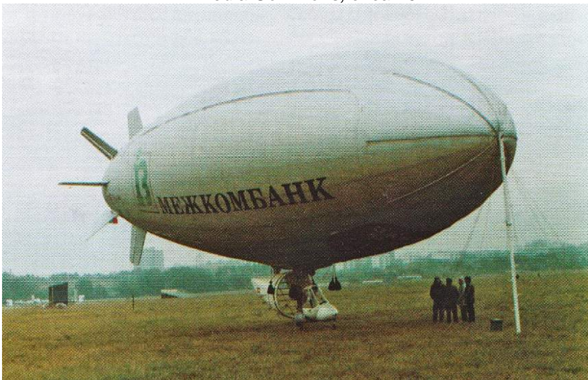
Aerostatica-01 sitting on its tricycle landing gear. Source: Boyko (2001)
