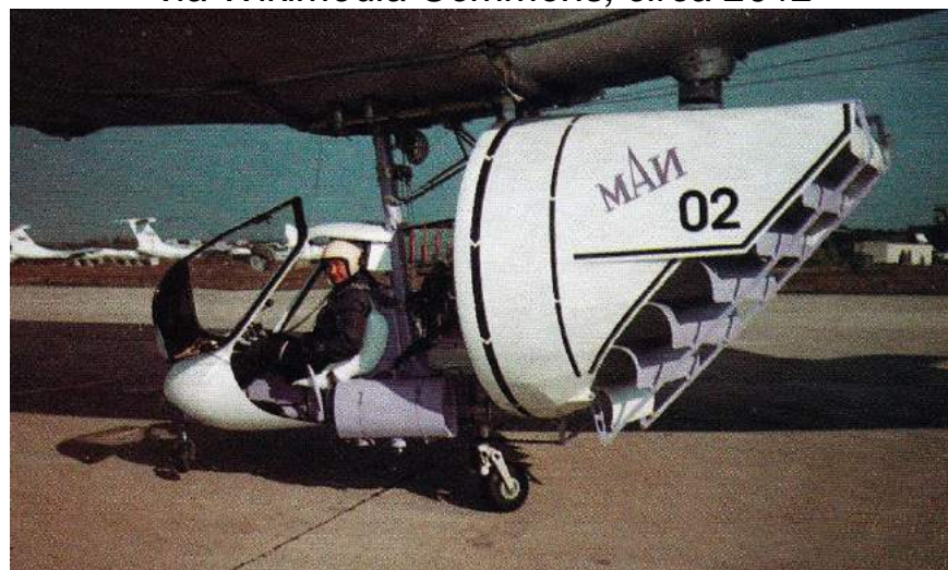
Shrouded propeller & thrust deflection louvers. Source: Boyko (2001)
