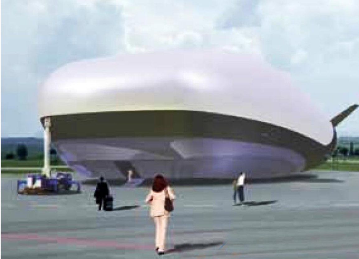
Rendering of the luxury cruising airship boarding thru a bow door. Note that a mobile mooring mast is connected. Source: Bauhaus Luftfahrt (Yearbook 2008)
