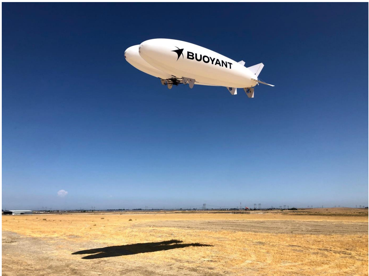
Buoyant Aero's 20 ft (6.1 m) subscale demonstrator in flight. Source: Buoyant Aero
