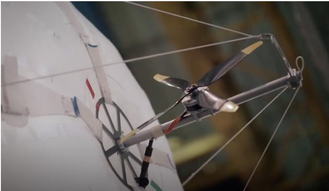
The two main electric motor-driven propellers are attached to the non-rigid envelope with straps and cables secured to reinforced areas of the envelope. Source: Screenshot from RTE video (Dec 2020)
