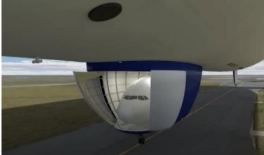
A large cargo bay with clamshell doors under the gas envelope provides easy loading and unloading. Source, above: screenshot from Altran Aerospace video, below: rendering by Bernard Guillaume
