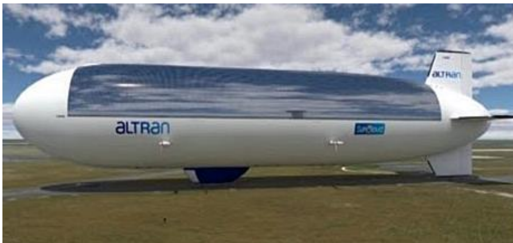
Sun Cloud profile view. Note the large solar array on the top of the hull. Source: screenshot from Altran Aerospace video (2013)
