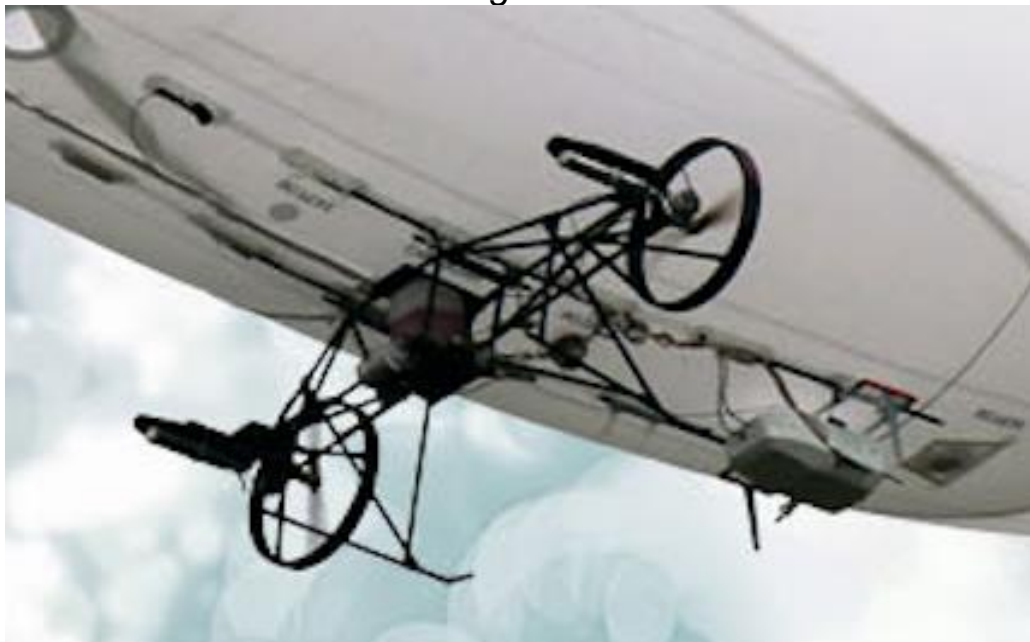
Close-up of DP-29 propulsion and payload modules, attached to the envelope via twin rails supported from reinforced areas of the envelope. Source: DKBA
