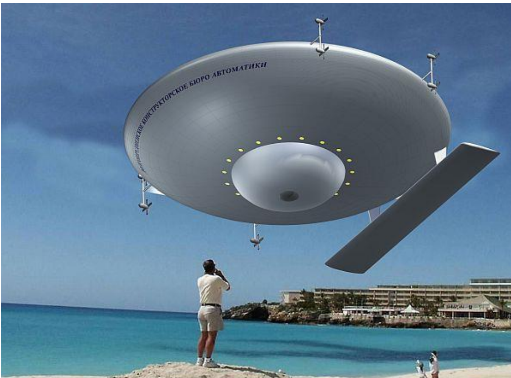
Rendering of an unmanned Aerocrat REP airship. Note the large horizontal stabilizer at the stern; a common feature on lenticular airships. Source: DKBA via LiveJournal (25Jan2009)
