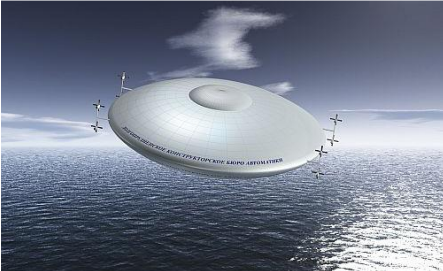
Rendering of an Aerocrat REP airship in flight. Note the four sets of two electrically-driven propellers along the flanks of the airship. Source: DKBA via LiveJournal (25Jan2009)
