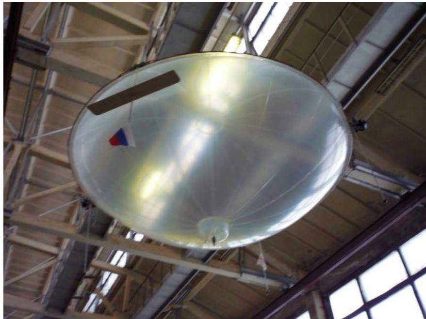
Demonstrator flying inside the DKBA boathouse. Note the relatively small, black horizontal stabilizer. Source, both photos: DKBA via LiveJournal (25Jan2009)
