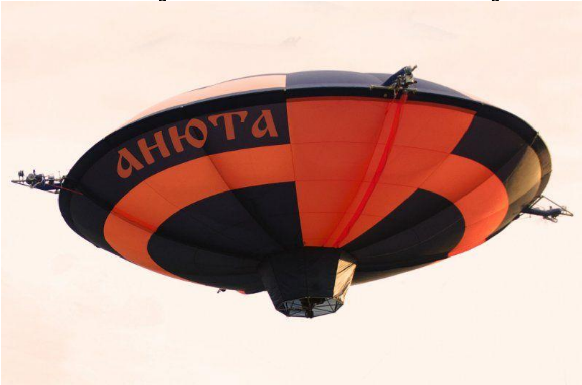
DP-27 in free flight. Three of four vectored propellers are visible. Source, both photos: DKBA
