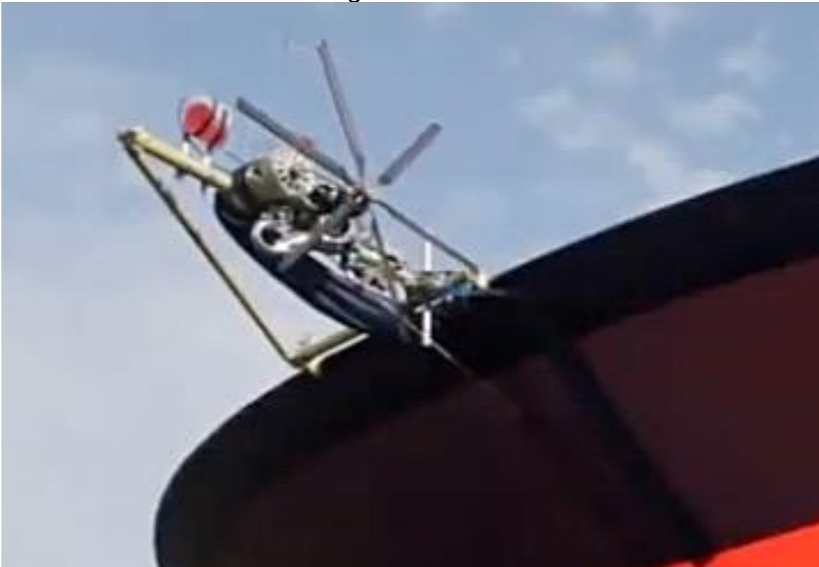
DP-27 vectored propeller (1 of 4). Source, both photos: DKBA
