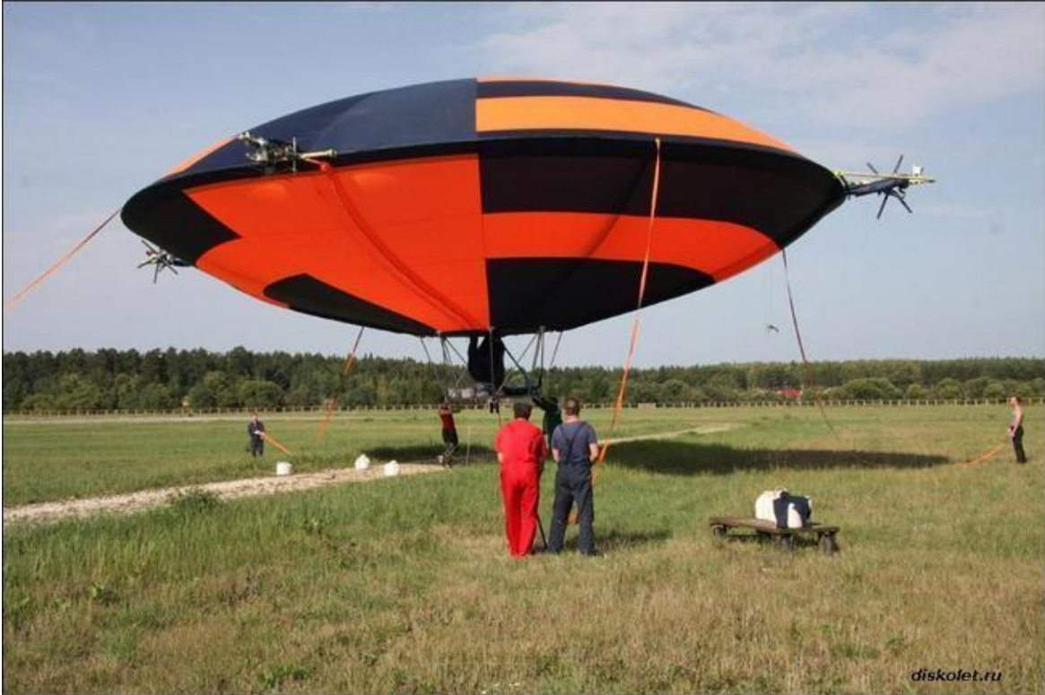
DP-27 tethered with gondola exterior skin removed.
