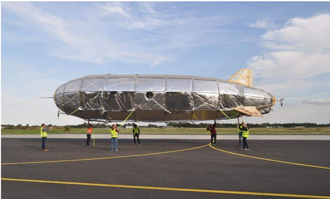
FlyWin subscale demonstrator airship moving out of its hangar and conducting the outdoor float test. Source: Colin Delfosse photos via detours (12 April 2019)
