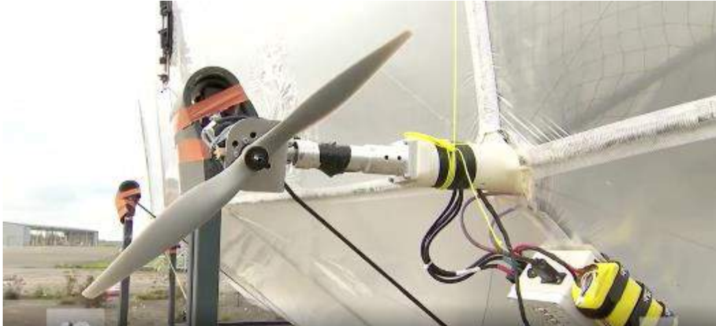
FlyWin demonstrator flank propeller, supported from a node in the rigid composite frame. Source: Screenshot from LinkedIn video
