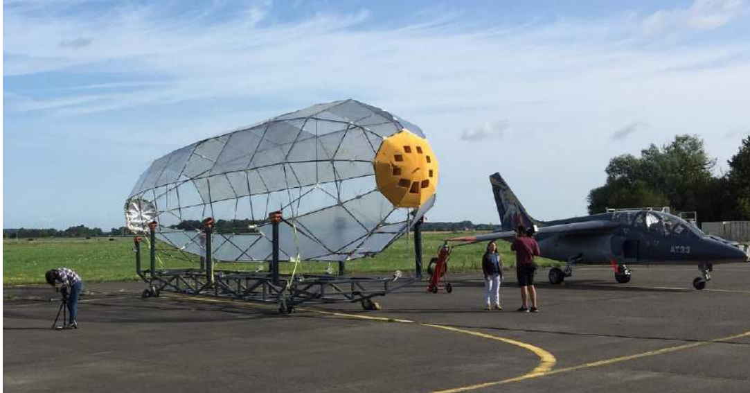
FlyWin demonstrator in its cradle, bow quarter view, with bow propeller removed. Source: FlyWin SA
