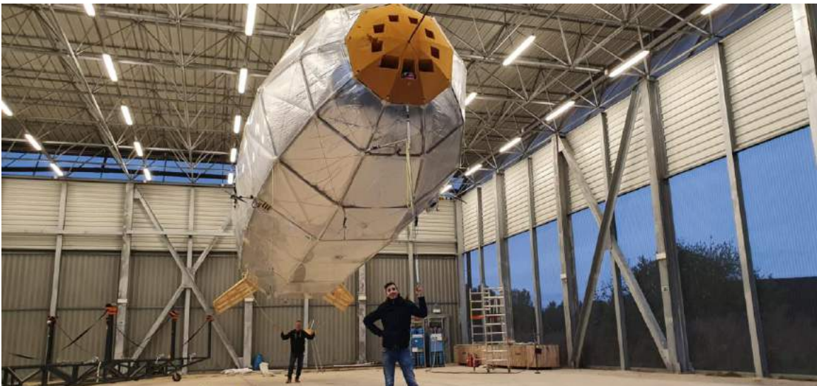
FlyWin subscale demonstrator airship indoor float test. Source, both photos: FlyWin SA
