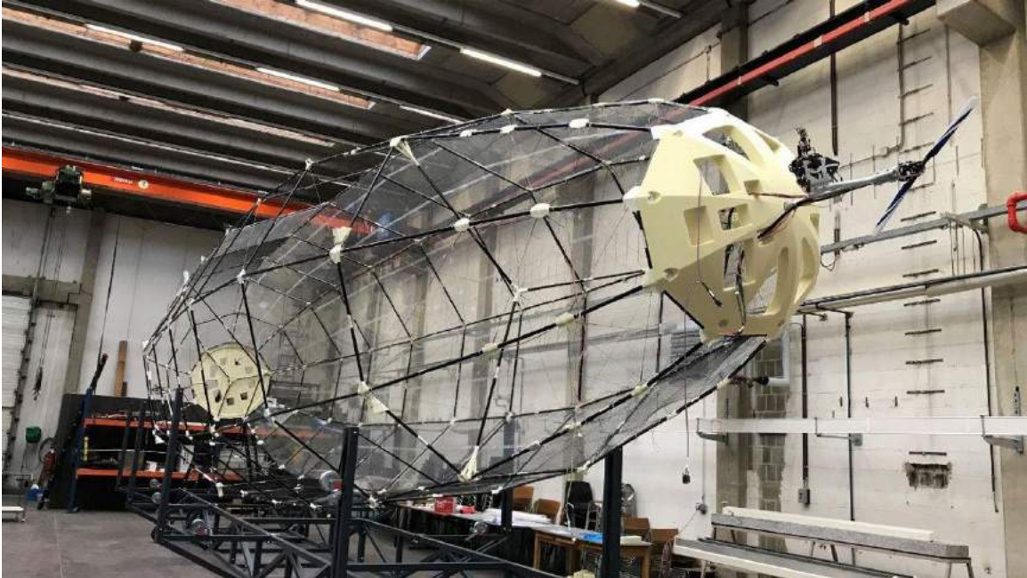
FlyWin subscale demonstrator airship during construction. Note the nose and tail caps attached to the carbon composite tubular rigid airframe. Source: RTBF - Erik Dagonnier (8 March 2018)
