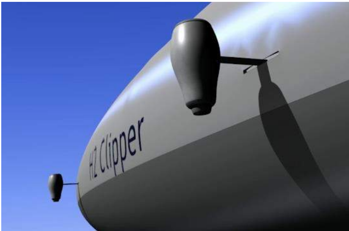
Vectored high-bypass ratio turbofan engines burn gaseous hydrogen fuel. Source, both graphics: H2 Clipper, Inc.
