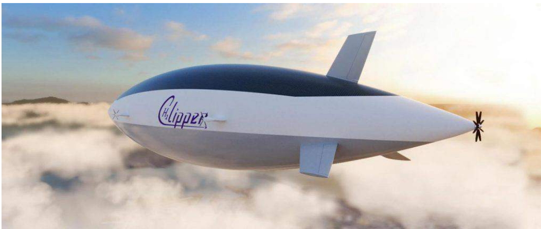
H2 Clipper viewed from the stern quarter. Note the inverted-Y tailplanes and tail-mounted propeller.
