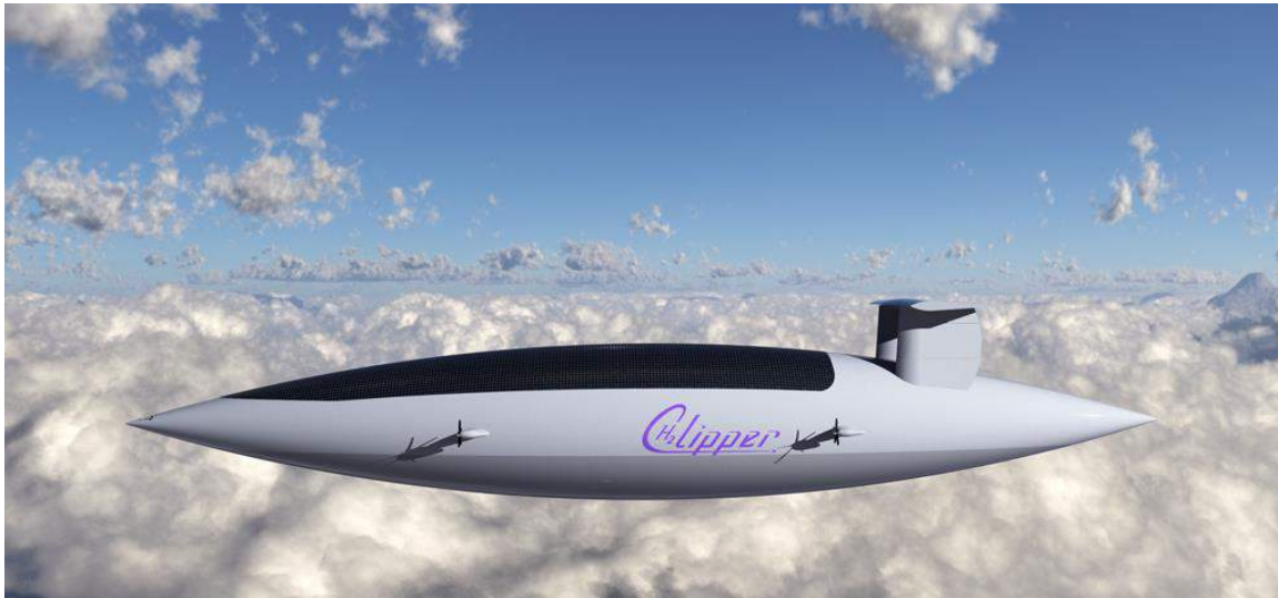
H2 Clipper profile view. Note the large, flank-mounted propellers. Source: H2 Clipper, Inc. (circa 2020)
