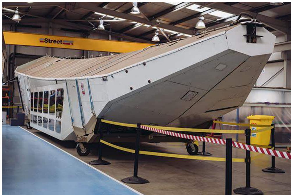
Original prototype's rigid gondola at the HAV facility in Bedford. Source: Tom Jamieson via Financial Times (11 October 2019)
