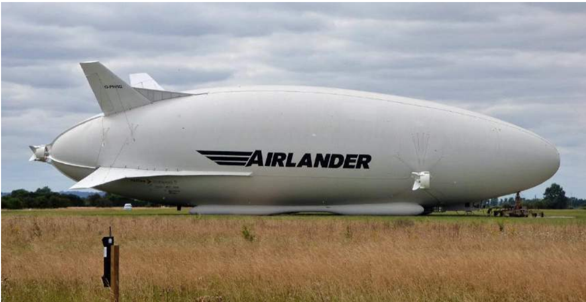
Profile view of the Airlander 10 prototype sitting on its inflated skids before first flight. Source: The Airship Heritage Trust
