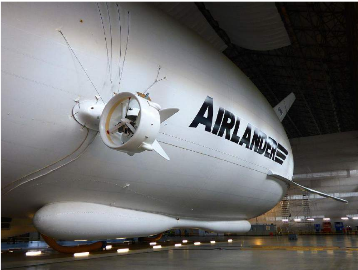
Close-up view of the assembled Airlander 10 prototype in 2016 showing a flank-mounted vectored-thrust propulsor and one of the landing skids. Source: Philbobagshot / Wikipedia
