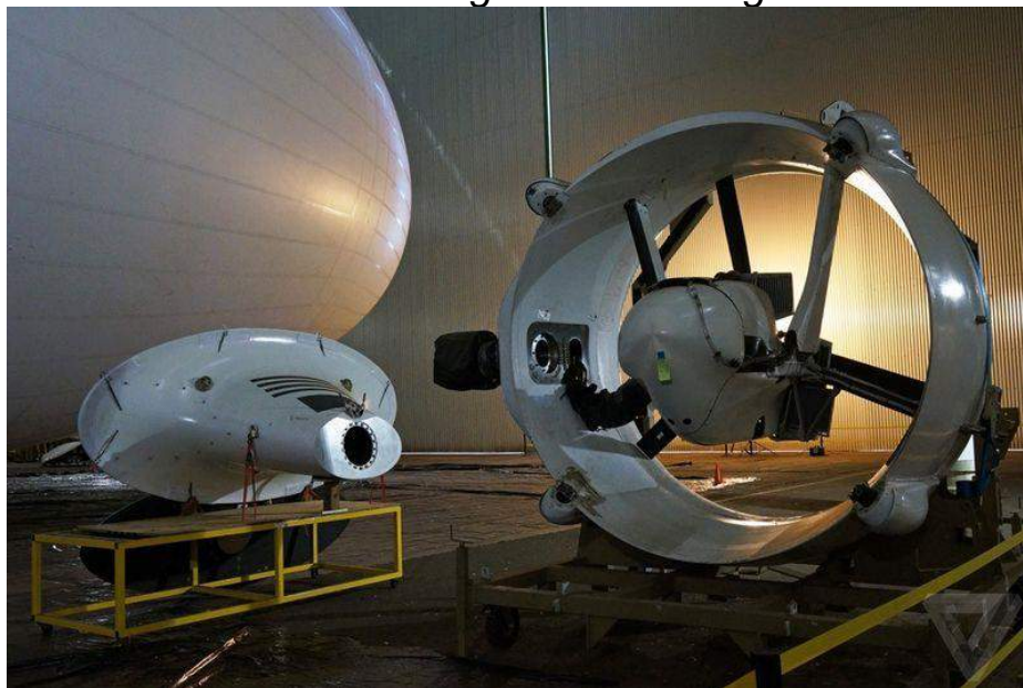
One of the flank-mounted diesel-powered vectoring thrusters. Source, both photos: The Verge, 8 July 2014
