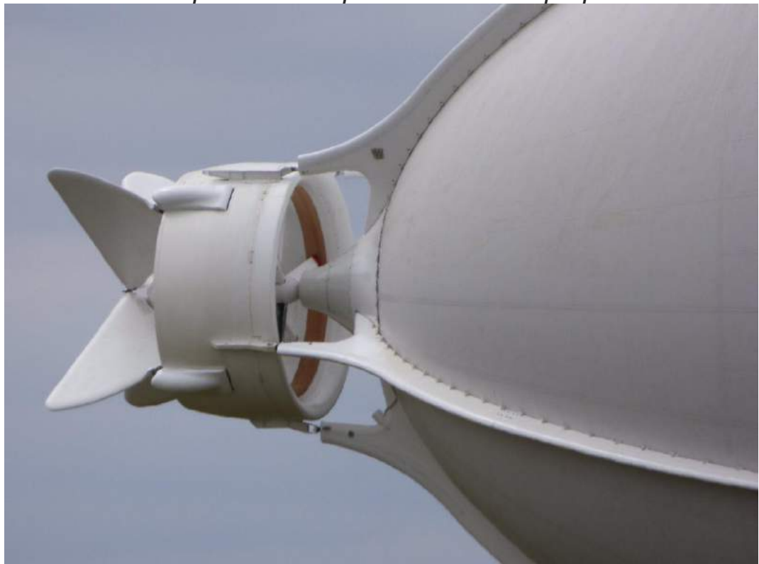
Close-up of one stern propulsor. Source, both photos: The Airship Heritage Trust
