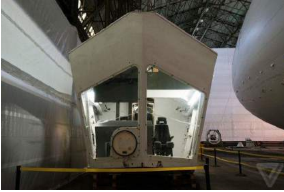
Left: The cockpit is at the front of the elongated payload module suspended under the centerline of the gas envelope.
