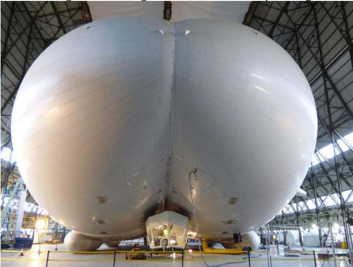
Bow-on view of the Airlander 10 prototype sitting on its inflated skids in Hangar 1 at Cardington with the rigid mission module being attached to the aeroshell. Source: Philbobagshot / Wikipedia
