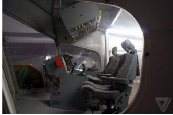
Left: The cockpit is at the front of the elongated payload module suspended under the centerline of the gas envelope.
