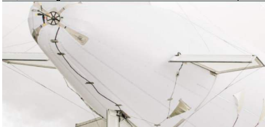
The vertical and horizontal tail fins have moving aerodynamic control surfaces. A small propeller attached at the tail with straps and cables provides lateral thrust to improve low-speed handling. Source: CNIM Air Space
