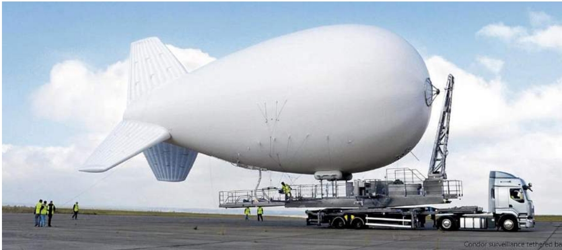
Condor on its mobile mooring platform with tractor trailer.
