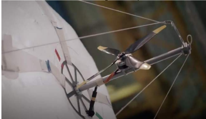
The two main electric motor-driven propellers are attached to the non-rigid envelope with straps and cables secured to reinforced areas of the envelope. Source, two images above: Screenshots from RTE video (Dec 2020)
