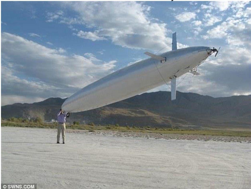
Police technician handles the HB50 on the ground. Note the thrust vectoring stern-mounted propeller. Source: SWNS.com via Daily Mail
